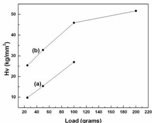
Fig.11 Vickers Hardness of (a)  $\gamma$ -glycine (b)  $\text{AgNO}_3$  doped  $\gamma$ -glycine
