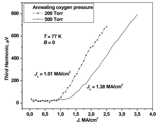
Fig. 3. Dependence of the third harmonic response signal amplitude on the screening current density  $J$  induced in YBCO films at 77 K by an AC magnetic field ( $<5$  mT). The third harmonics of the response signal arise at  $J = 1$  MA/cm $^2$  and  $J = 1.4$  MA/cm $^2$ , which correspond to the critical current densities of the samples annealed at 200 and 500 Torr respectively.
