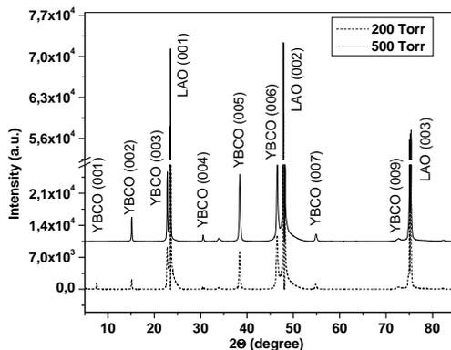
Fig. 2. X-ray diffraction pattern for YBCO films annealed at 200 and 500 Torr oxygen pressures.
