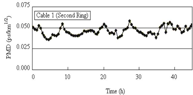
Fig. 4. Variation of PMD with ambient temperature change observed in the second ring of Cable 1
