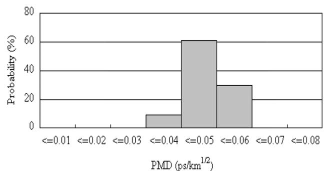
Fig. 6. Distribution of PMD values in the second ring of Cable 1
