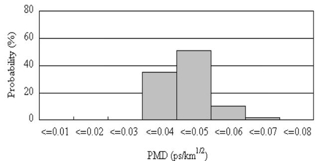
Fig. 5. Distribution of PMD values in the first ring of Cable 1
