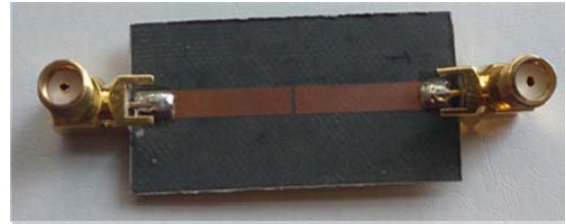
Fig. 9. Fabricated bandpass filter, front view
