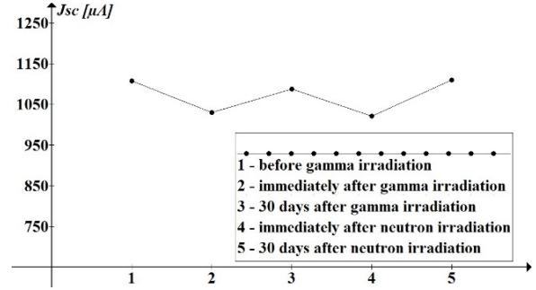
Fig. 4. Short-circuit current of the solar panels before and after gamma and neutron irradiation
