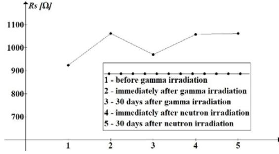
Fig. 2. Series resistance of the solar panels before and after gamma and neutron irradiation
