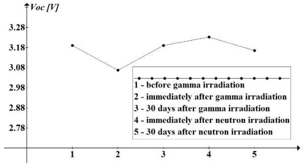
Fig. 5. Open-circuit voltage of the solar panels before and after gamma and neutron irradiation
