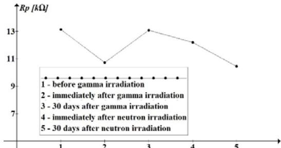
Fig. 3. Parallel resistance of the solar panels before and after gamma and neutron irradiation
