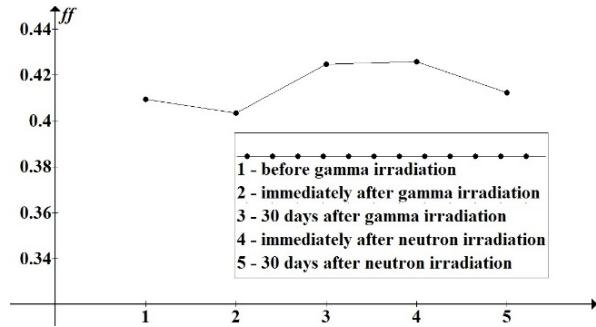
Fig. 6. Fill factor of the solar panels before and after gamma and neutron irradiation
