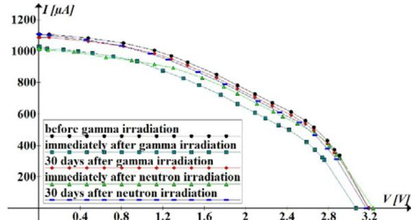
Fig. 1. I-V characteristics of the solar panels before and after gamma and neutron irradiation.
