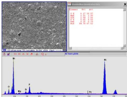
Fig. 3. EDX diagram showing the chemical composition of the composite layer deposited (NiP + 120 g / l talc)
