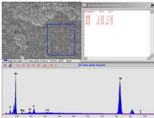
Fig. 2. EDX diagram showing the chemical composition of the composite layer deposited (NiP + 40 g / l talc)
