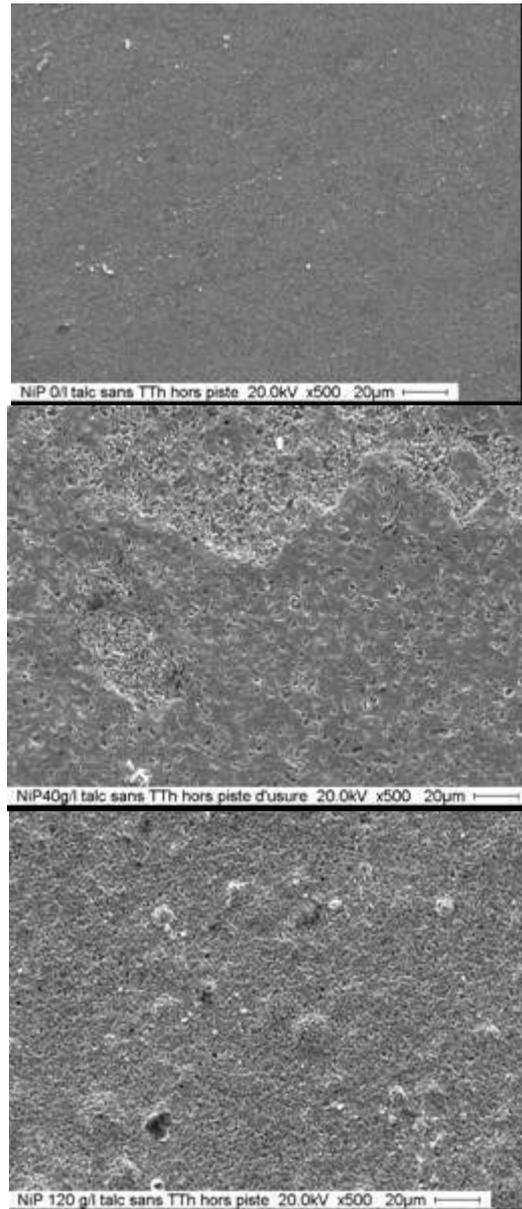
Fig. 5. Different deposit morphologies (SEM micrographs, magnification  $\times 500$ ): a - NiP without talc, b - NiP + 40 g/l talc, c - NiP + 120 g/l talc
