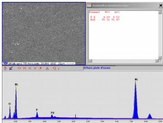
Fig. 1. EDX diagram showing the chemical composition of the composite layer deposited (NiP without talc)
