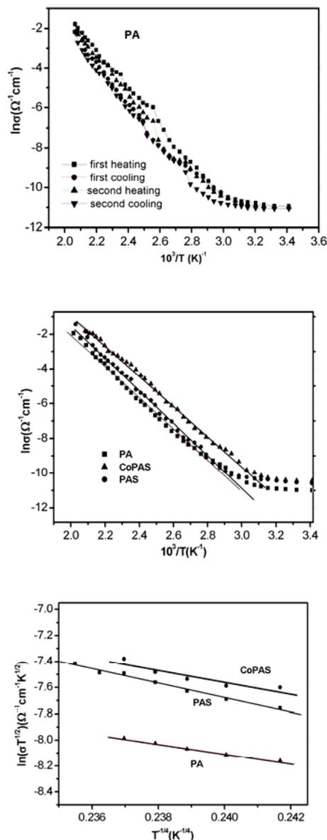
Fig.4. The electrical conductivity as a function of temperature: a) Temperature dependence during heat treatment; b)  $\ln\sigma = f(10^3/T)$  plots, intrinsic domain; c)  $\ln(\sigma T^{1/2}) = f(T^{-1/4})$  plots, extrinsic domain
