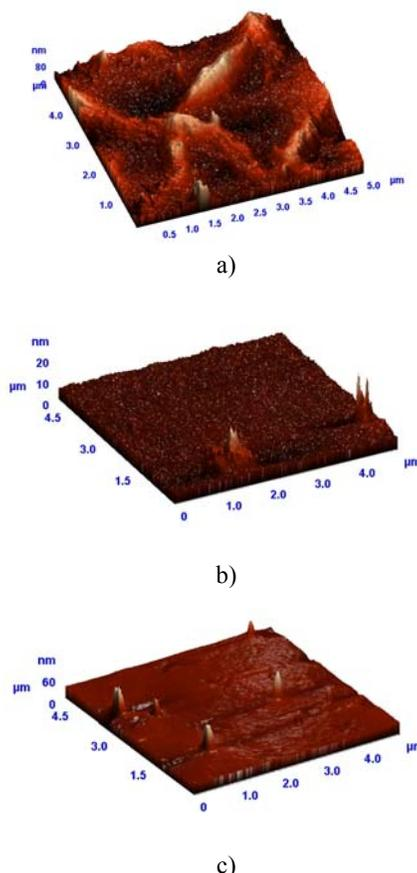
Fig. 2.  $5 \times 5 \mu\text{m}$  AFM images of thin films: a) PA b) CoPAS, c) PAS
