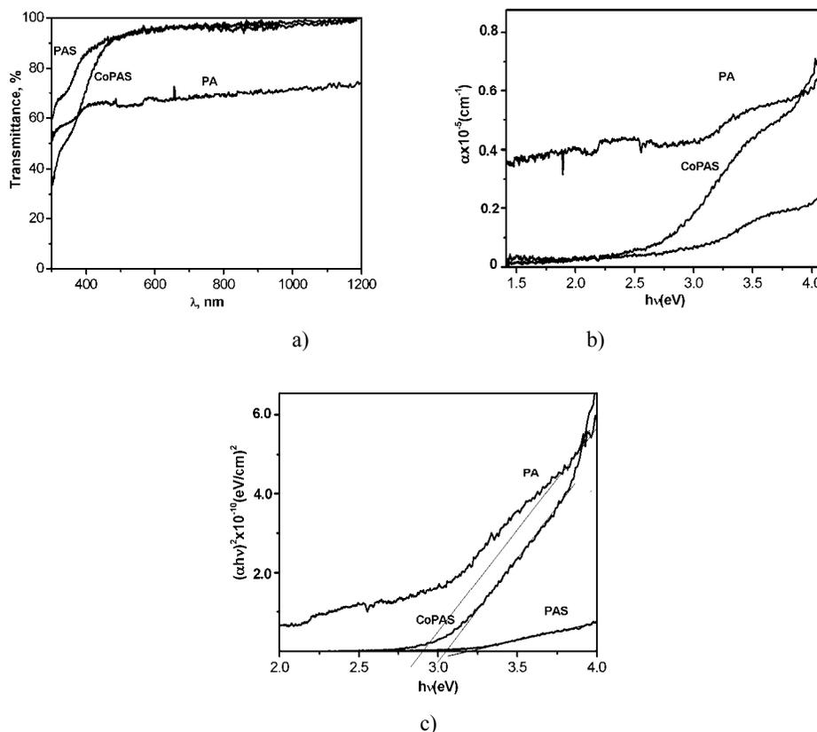
Fig. 3. Thin film optical spectra: a) Transmittance spectra; b) Absorption coefficient; c) Linear approximation of absorption edges of thin films
