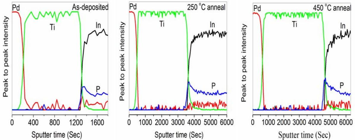
Fig. 4. Auger depth profile of the Pd/Ti Schottky contact to n-InP: (a) as-deposited, (b) annealed at 250 °C and (c) annealed at 450 °C
