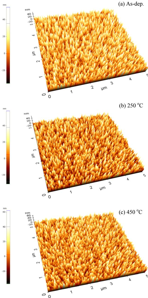
Fig. 6. AFM micrographs of the Pd/Ti Schottky contacts to n-InP: (a) as-deposited, (b) annealed at 250 °C and (c) annealed at 450 °C
