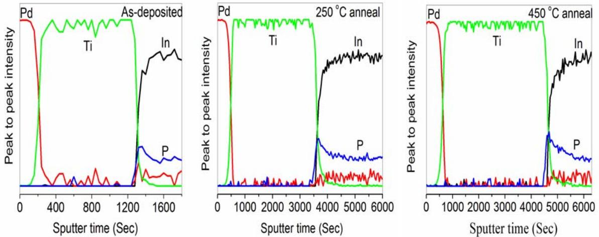
Fig. 4. Auger depth profile of the Pd/Ti Schottky contact to n-InP: (a) as-deposited, (b) annealed at 250 °C and (c) annealed at 450 °C
