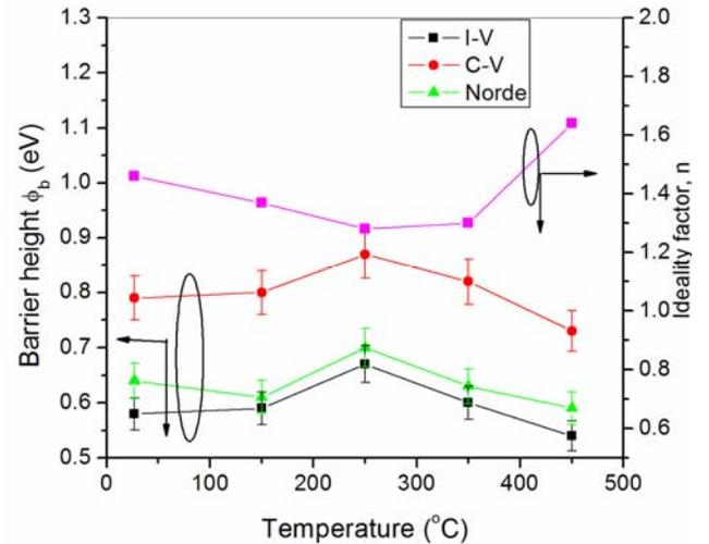
Fig. 3. Effective barrier height and ideality factor of Pd/Ti/n-InP diodes after annealing for 1 min at different temperature.
