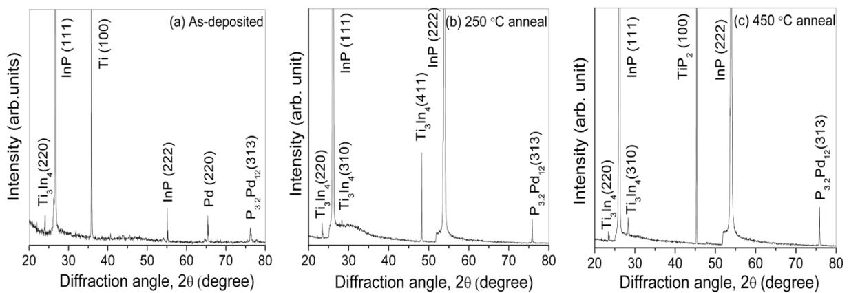
Fig. 5. XRD plots of the Pd/Ti/n-InP Schottky diode: (a) as-deposited, (b) annealed at 250 °C and (c) annealed at 450 °C.
