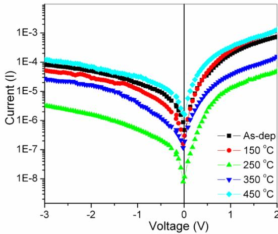
Fig. 1. Typical I-V characteristics of Pd/Ti Schottky contacts to n-InP as a function of annealing temperature
