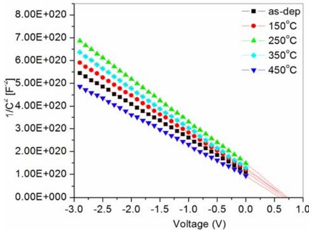
Fig. 2. Plot of  $1/C^2$  versus  $V$  for Pd/Ti Schottky contacts to n-InP annealed at different temperature
