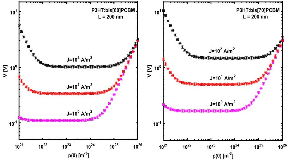
Fig. 4. Theoretical results of voltage versus the boundary carrier density of electron-only devices based on the P3HT:bis[60]PCBM and P3HT:bis[70]PCBM. Different Lines correspond to different current density (color online)
