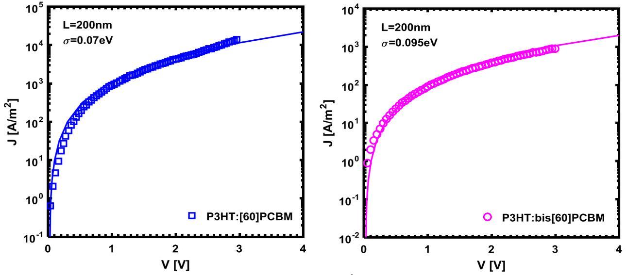
Fig. 2.  $J$ - $V$  characteristics of electron-only devices for P3HT:[60]PCBM and P3HT:bis[60]PCBM. Symbols are experimental data from Ref. [14], lines are the numerically calculated results from Eqs. (1)~(6)
