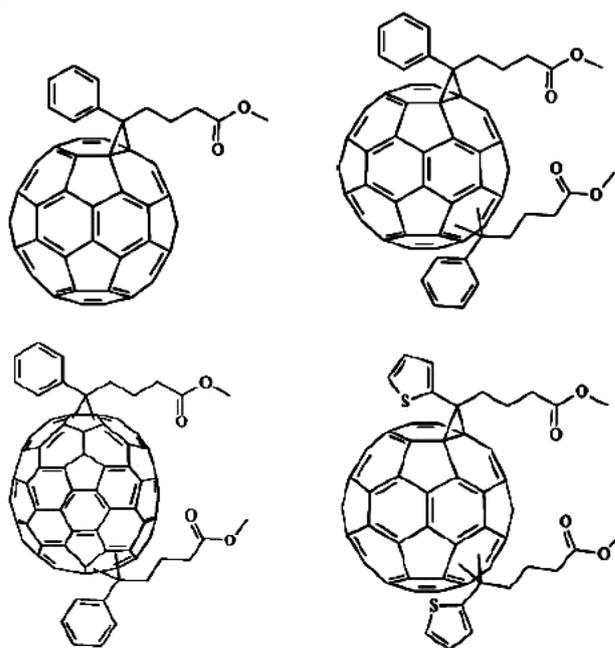
Fig. 1. Chemical structures of materials used in this study. From top left to bottom right, [60]PCBM, and highly generalized structures for the isomeric mixtures of the bis[60]PCBM, bis[70]PCBM and bis[60]ThCBM
