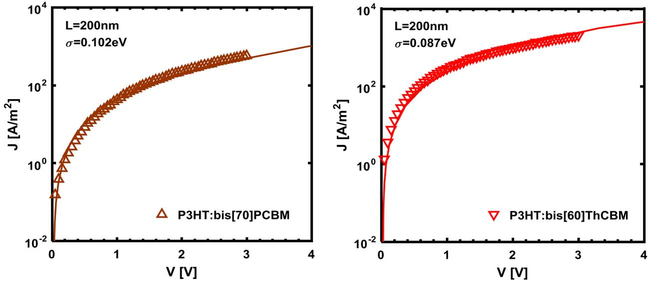
Fig. 3.  $J$ - $V$  characteristics of electron-only devices for P3HT:bis[70]PCBM and P3HT:bis[60]ThCBM. Symbols are experimental data from Ref. [14], lines are the numerically calculated results from Eqs. (1)~(6) (color online)
