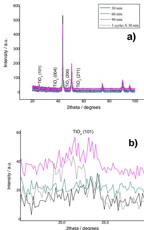
Fig. 1. X-ray diffraction profiles of a) deposited and annealed at 400 °C TiO<sub>2</sub> films coated 316L SS and b) a zoomed TiO<sub>2</sub> peak for (101) crystallographic plane.
