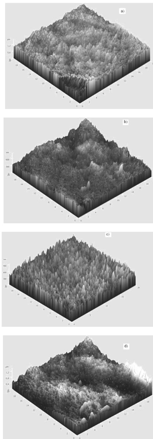
Fig. 3. AFM images of  $\text{TiO}_2$  films at different stages of deposition: (a) 30 min; (b) 60 min; (c) 90 min and (d) 3 consecutive cycles of 30 min each
