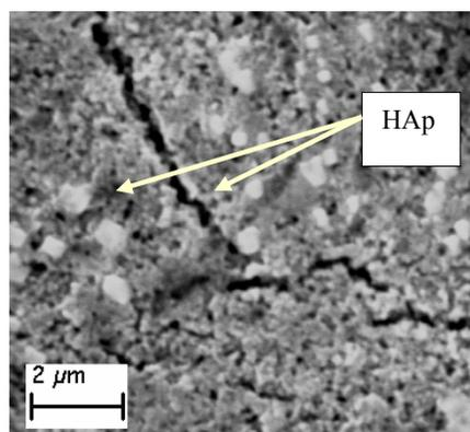
Fig. 4. The surface morphology of HAp growth after 21 days of immersion in SBF
