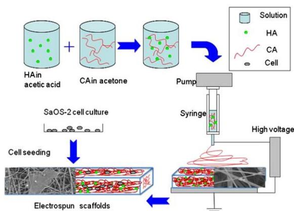
Fig. 4. Schematic of the electrospinning and cell culture process used to obtain 3D cell seeded scaffolds. Insets are SEM micrographs revealing cross sectional views of the scaffolds before and after the cell seeding process. Reprinted with permission from [73] ©2013 Elsevier B.V.
