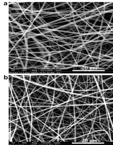
Fig. 3. SEM images of electrospun fibers PLA-F (a) and AHC-PLA-F (b). Reprinted with permission from [57]. ©2013 Elsevier B.V.
