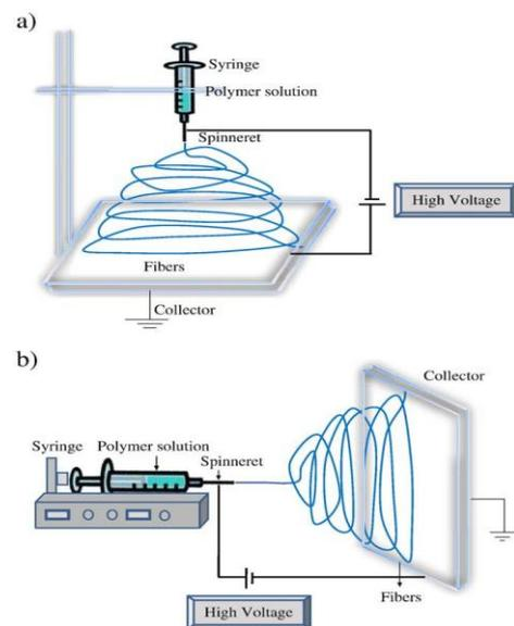
Fig. 1. Schematic diagram of set up of electrospinning apparatus (a) typical vertical set up and (b) horizontal set up of electrospinning apparatus. Reprinted with permission from [11]. ©2013 Elsevier B.V.
