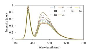
Fig. 4. The emission spectra of 6600 K WLEDs as a function of SrBaSiO4:Eu<sup>2+</sup> concentration
