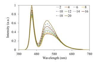
Fig. 6. The emission spectra of 7700 K WLEDs as a function of SrBaSiO4:Eu<sup>2+</sup> concentration
