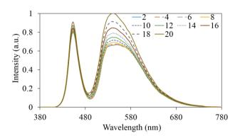
Fig. 3. The emission spectra of 5600 K WLEDs as a function of SrBaSiO4:Eu<sup>2+</sup> concentration
