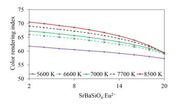
Fig. 10. The color rendering index of WLEDs as a function of SrBaSiO<sub>4</sub>:Eu<sup>2+</sup> concentration
