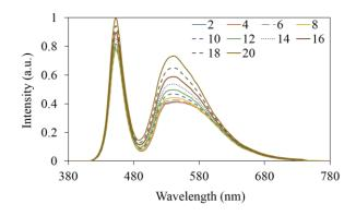
Fig. 5. The emission spectra of 7000 K WLEDs as a function of SrBaSiO4:Eu<sup>2+</sup> concentration
