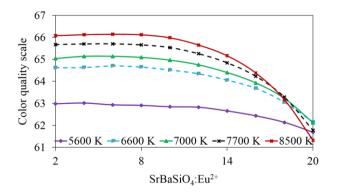
Fig. 11. The color quality scale of WLEDs as a function of SrBaSiO4:Eu<sup>2+</sup> concentration
