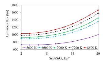
Fig. 8. The luminous flux of WLEDs as a function of SrBaSiO4:Eu<sup>2+</sup> concentration
