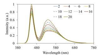
Fig. 7. The emission spectra of 8500 K WLEDs as a function of SrBaSiO4:Eu<sup>2+</sup> concentration
