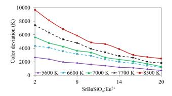
Fig. 9. The color deviation of WLEDs as a function of SrBaSiO4:Eu<sup>2+</sup> concentration
