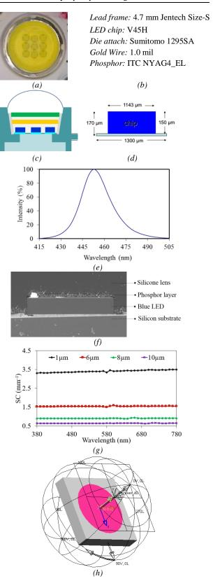
Fig. 1. Photograph of WLEDs structure: (a) Actual WLEDs, (b) its parameters, (c) Illustration of doublelayer phosphor model, (d) Side view of blue chip,(e) Emission spectrum of LED chip; (f) SEM image of WLEDs, (g) Scattering coefficient of SrBaSiO4:Eu<sup>2+</sup>, (h)Simulation of of WLEDs
