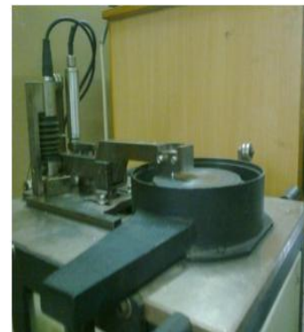
Fig. 2. Photographic view of the pin-on-disc wear-testing machine
