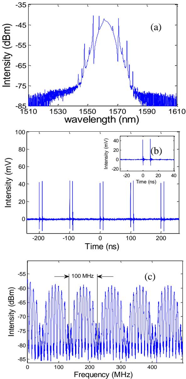
Fig. 4. (a) Optical spectrum for dual-soliton states with the temporal separation of 10 ns. (b) Oscilloscope traces. The upper right insert shows the pulses per round trip. (c) RF spectrum.
