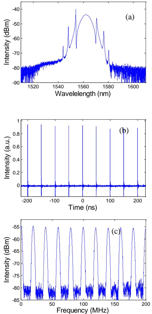
Fig. 7. The second harmonic mode locked mode of the proposed fiber laser, (a) Optical spectrum, (b) Oscilloscope trace, (c) RF spectrum.
