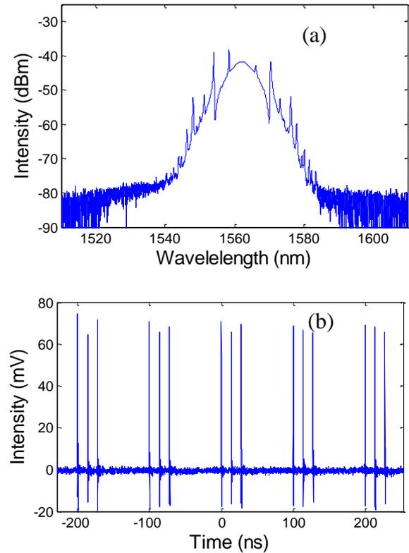
Fig. 5. The triple pulses operation state, (a) Optical spectrum for triple pulses states, (b) The corresponding oscilloscope traces.
