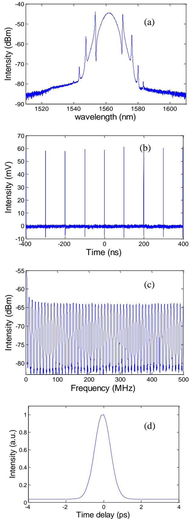
Fig. 2. (a) Optical spectrum, (b) Oscilloscope trace, (c) RF spectrum, and (d) Autocorrelation trace at the fundamental cavity frequency state.
