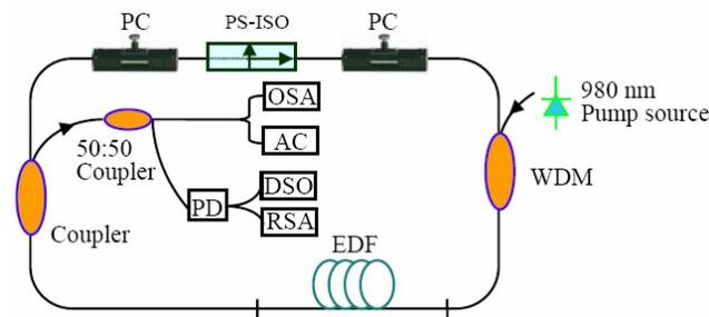
Fig. 1. Schematic diagram of the passively mode-locked ring fiber laser. PC: Polarization controller; WDM: Wavelength-division multiplexer; EDF: Erbium doped fiber; PS-ISO: Polarization sensitive isolator; PD: Photodetector; OSA: Optical spectrum analyzer; DSO: Digital storage oscilloscope; RSA: Radio frequency spectrum analyzer; AC: Autocorrelator.
