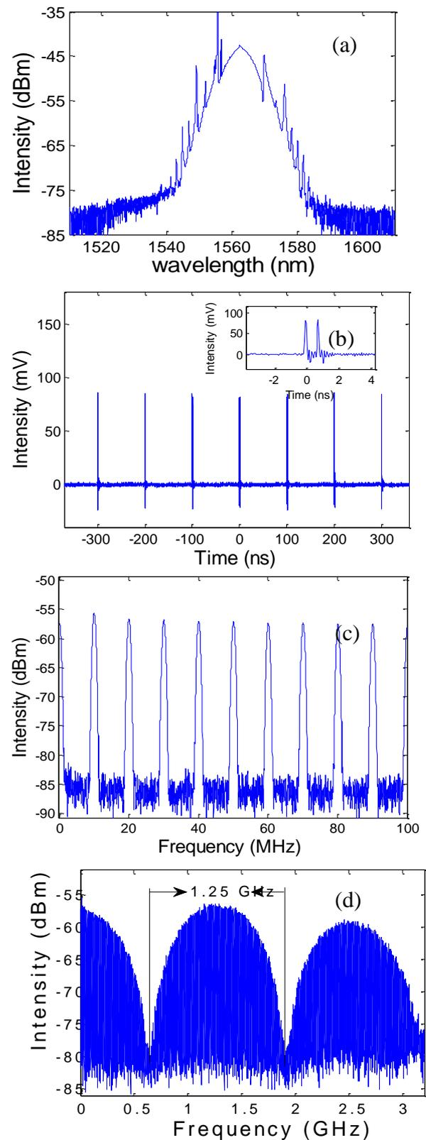
Fig. 3. (a) Optical spectrum for dual-soliton states with the temporal separation of 0.8 ns. (b) Oscilloscope traces. The upper right insert shows the pulses per round trip. The RF spectra are in different spans. Span: (c) 100 MHz, (d) 2 GHz.
