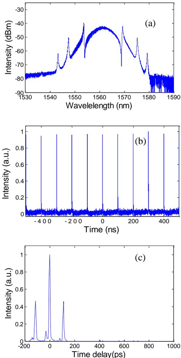
Fig. 6. The bound state of dual pulses operation states. (a) Optical spectrum, (b) Oscilloscope trace, and (c) Autocorrelation trace at the bound state of dual pulses operation states.
