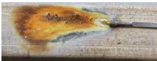
Fig. 5. The lead thread vaporized and ionized through modified pulse duration.
