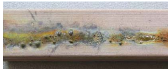
Fig. 2. The lead sample vaporized and ionized.
