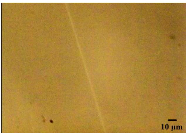
Fig.3. Optical micrograph of the perpendicular recording waveguide line in GGA15 glass.
