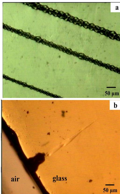
Fig.2. Optical micrographs of the perpendicular recording geometry in GGB10 glass (a) and the parallel recording geometry in GGA15 glass (b).
