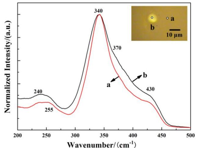
Fig.5. Micro-Raman spectra of GGA15 glass before (a) and after (b) laser irradiation.
