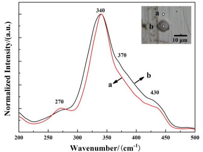
Fig.4. Micro-Raman spectra of GGB10 glass before (a) and after (b) laser irradiation.
