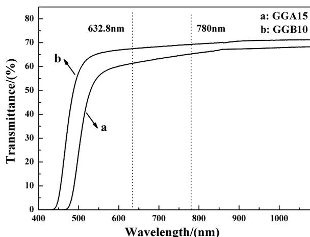
Fig.1. Optical transmission spectra of the as-prepared GGB10 and GGA15 glasses in the Vis-NIR region.
