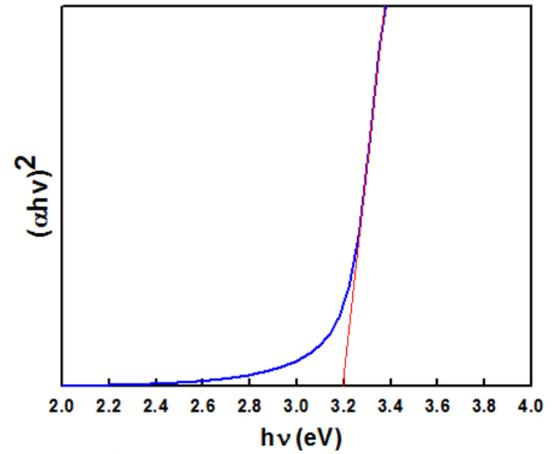
Fig. 4.  $(\alpha h\nu)^2$  versus photon energy ( $h\nu$ ) of ZnO thin film on glass substrate by using RF sputtering method.
