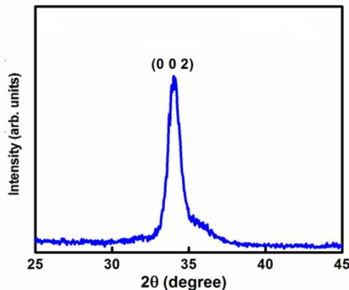
Fig. 2. X-ray diffraction pattern of ZnO thin film deposited on  $p$ -type Si  $\langle 100 \rangle$  substrate by using RF sputtering process
