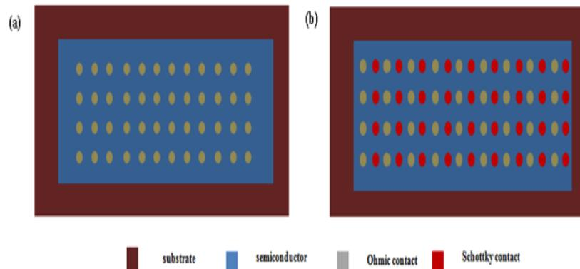
Fig. 1. (a) Schematic of ZnO based photoconductor (b) ZnO based photo-diode.
