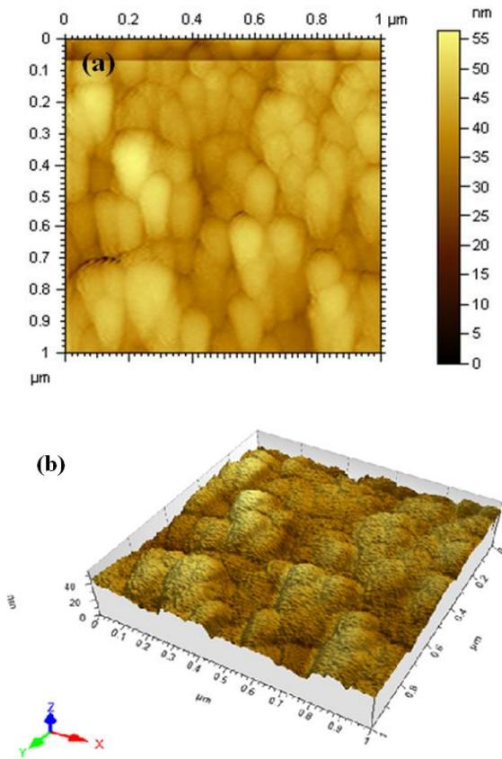
Fig. 3. AFM images of ZnO thin film on p-type Si <100> substrate by RF sputtering process (a) 2-D image (b) 3-D image
