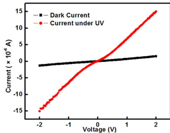
Fig. 5.  $I$ - $V$  characteristics of the fabricated Al/ZnO/Al photo-conductor measured in dark and under illumination from -2 V to +2 V
