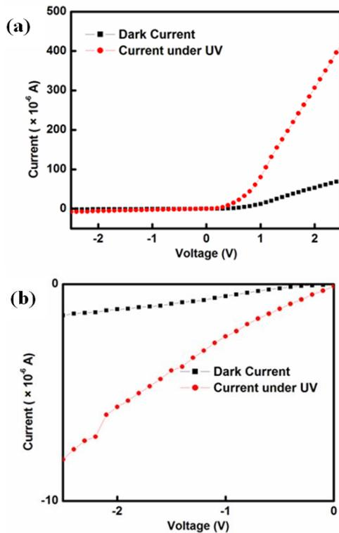
Fig. 6.  $I$ - $V$  characteristics of the fabricated Pd:Au/ZnO/Al photodetector measured in dark and under illumination (a) from -2 V to +2 V (b) in reverse bias condition
