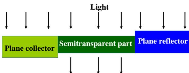
Fig. 7. Simplified prototype of the semitransparent solar thermoelectric cell
