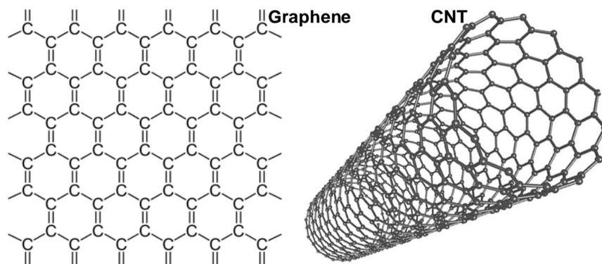
Fig. 1. Schematic diagrams of the two-dimensional graphene[18] and the carbon nanotubes (CNTs) [19]
