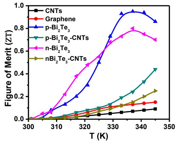
Fig. 6. Figure of merit (ZT) and temperature (T) relationships for the samples of composites of adhesive with CNTs, graphene, p-Bi<sub>2</sub>Te<sub>3</sub>, n-Bi<sub>2</sub>Te<sub>3</sub>, p-Bi<sub>2</sub>Te<sub>3</sub>-CNTs, and n-Bi<sub>2</sub>Te<sub>3</sub>-CNTs
