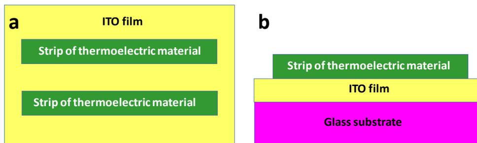
Fig. 2. The schematic diagrams of the top view (a) and front view (b) of the thermoelectric cells
