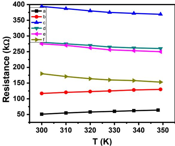
Fig. 4. Resistance-temperature relationships for the composites of adhesive with: CNTs (a), graphene (b), p-Bi<sub>2</sub>Te<sub>3</sub>(c), n-Bi<sub>2</sub>Te<sub>3</sub> (d), p-Bi<sub>2</sub>Te<sub>3</sub>-CNTs (e), n- Bi<sub>2</sub>Te<sub>3</sub>-CNTs (f)
