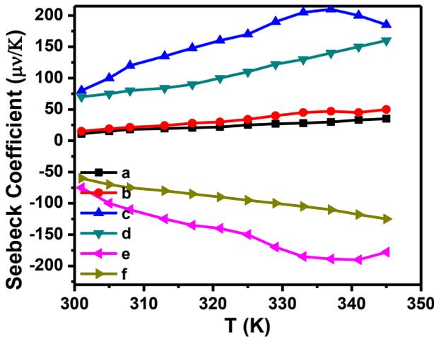
Fig. 5. Seebeck coefficient and temperature (T) relationships for the composites of adhesive with: CNTs (a), graphene (b), p-Bi<sub>2</sub>Te<sub>3</sub> (c), p-Bi<sub>2</sub>Te<sub>3</sub>-CNTs(d), n- Bi<sub>2</sub>Te<sub>3</sub>(e) and n-Bi<sub>2</sub>Te<sub>3</sub>-CNTs (f)
