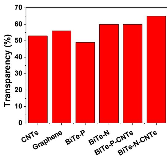
Fig. 3. Transparency of the CNTs, grapheme,  $p\text{-Bi}_2\text{Te}_3$ ,  $n\text{-Bi}_2\text{Te}_3$ ,  $p\text{-Bi}_2\text{Te}_3\text{-CNTs}$  and  $p\text{-Bi}_2\text{Te}_3\text{-CNTs}$  composite samples
