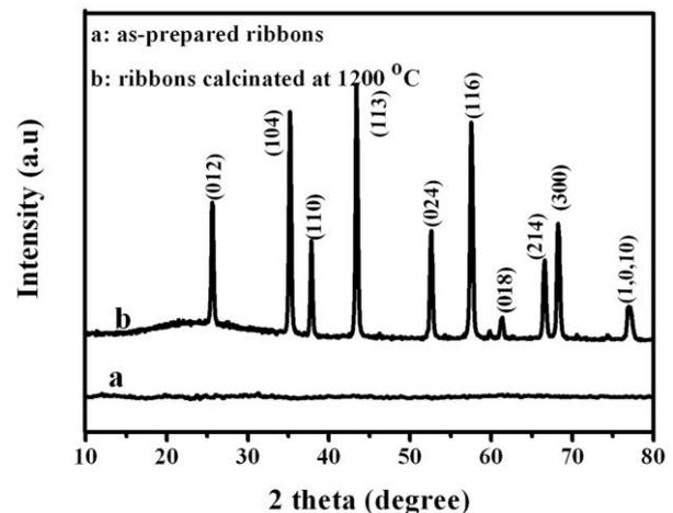
Fig. 2. XRD patterns of as-prepared ribbons and the ribbons after calcinated at 1200  $^{\circ}\text{C}$ .
