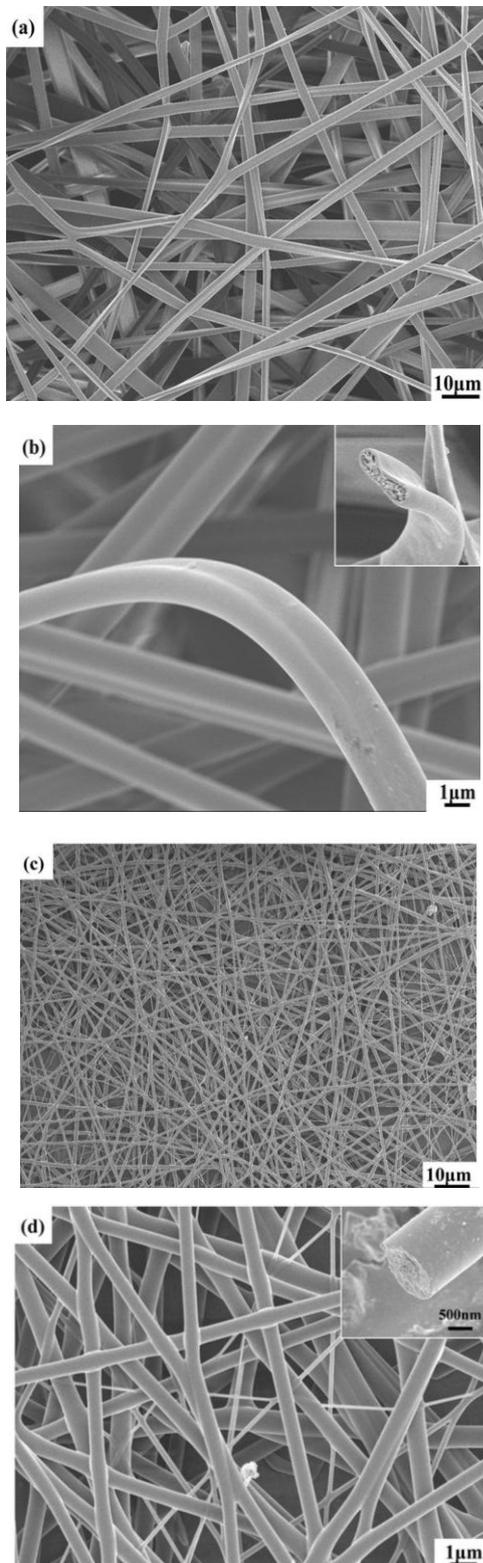
Fig. 1. SEM images of as-prepared fibers using mixed solvent (a), (b) and using ethanol only (c), (d). (a) in small magnification; (b) in high magnification and the cross section on the upright; (c) in small magnification; (d) in high magnification and the cross section on the upright.
