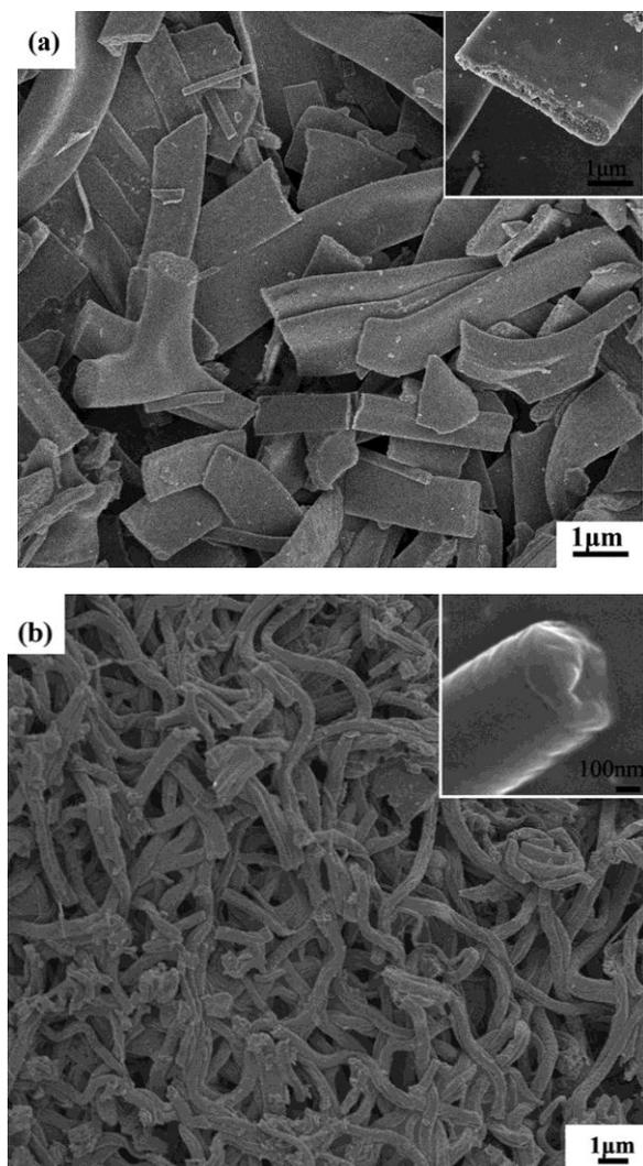
Fig. 3. SEM images of the fibers after calcinated at 1200 °C using mixed solvent (a) and using ethanol only (b).
