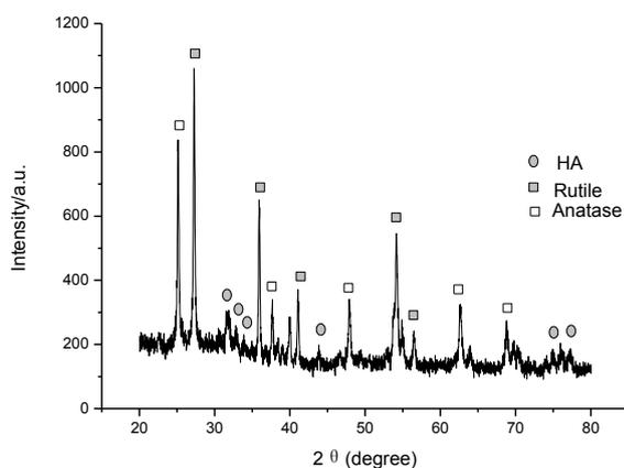
Fig. 4 XRD patterns of the  $\text{TiO}_2/\text{HA}$  composite coatings
