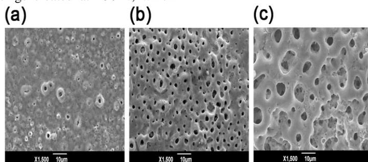
Fig. 1 Surface morphologies of the TiO<sub>2</sub> coatings formed at various applied voltages (MAO time is 5 min): (a) 200 V, (b) 300 V, (c) 450 V.
