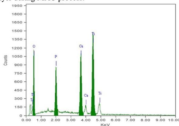
Fig. 2 EDS analysis of the TiO<sub>2</sub> coating formed in the Ca- and P-containing solution
