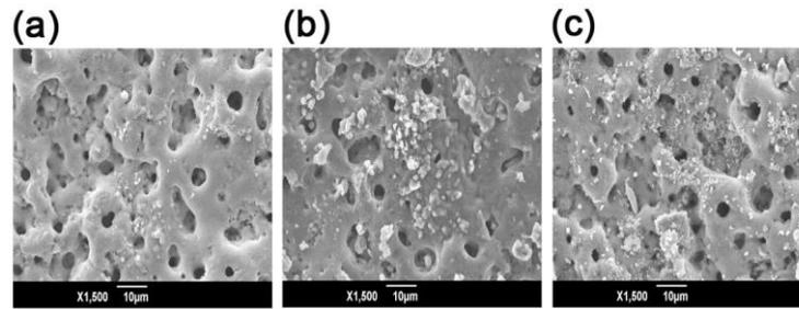
Fig. 3 Morphologies of biomimetic HA coating on the surface of  $\text{TiO}_2$  coating formed after immersing in SBF for different times: (a) 7 days, (b) 14 days, (c) 21 days.
