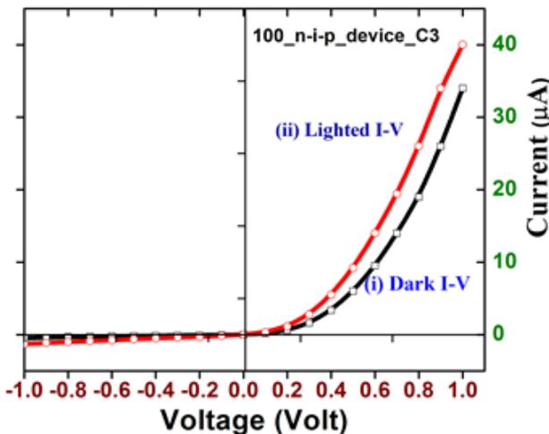
Fig. 4. Dark and lighted current-voltage (I-V) curve of 100\_n-i-p diode with circular top contact (color online)
