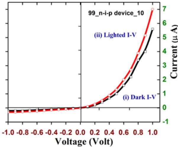
Fig. 3. Dark and lighted current-voltage (I-V) curve of 99\_Dev n-i-p diode with circular top contact (color online)
