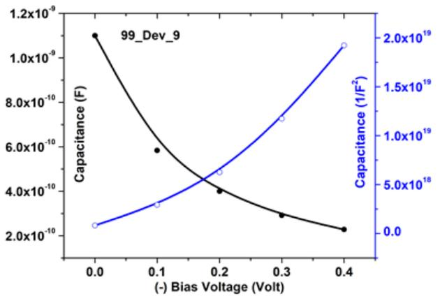
Fig. 5. Capacitance-voltage (C-V) curve of 99\_Dev\_9 n-i-p diode with circular top contact (color online)
