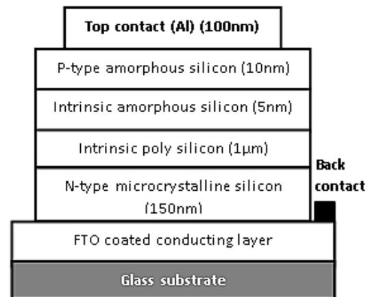
Fig. 1. 2D block diagram of HIT structured n-i-p diode
