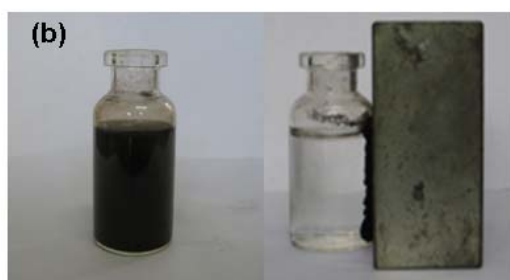
Fig. 8. Hysteresis loops of the \text{Fe}_3\text{O}_4/\text{MWNTs} nanocomposites measured at RT (a) and separation \text{Fe}_3\text{O}_4/\text{MWNTs} nanocomposites from solution under an external magnetic field (b).
