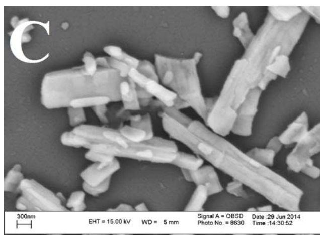
Fig. 7. SEM images of bismuth oxide samples, (A) without capping agent, (B) containing 3% PVA and (C) containing 5% PVA
