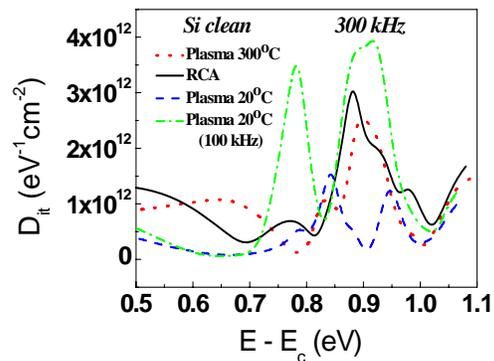
Fig. 2. Interface trap profiles in the Si bandgap.
