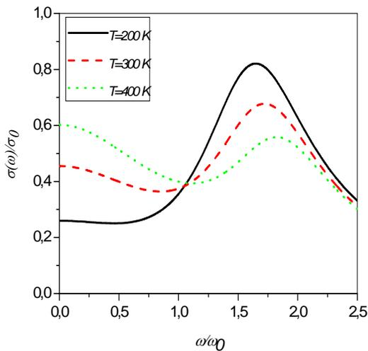
Fig. 4. Dependence of dynamic conductivity  $\sigma(\omega)$  with the frequency  $\omega$  for different values of  $T$  the other parameters are  $\Gamma=7$  and  $\xi=0.5$ .
