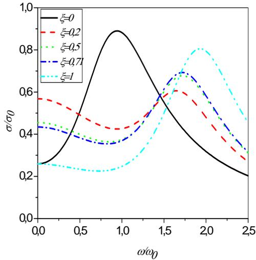
Fig. 3. Dependence of dynamic conductivity  $\sigma(\omega)$  with the frequency  $\omega$  for different values of  $\xi$ . The other parameters are  $\Gamma=7$ ,  $T=300$  K,  $V_1=0.1$  eV.
