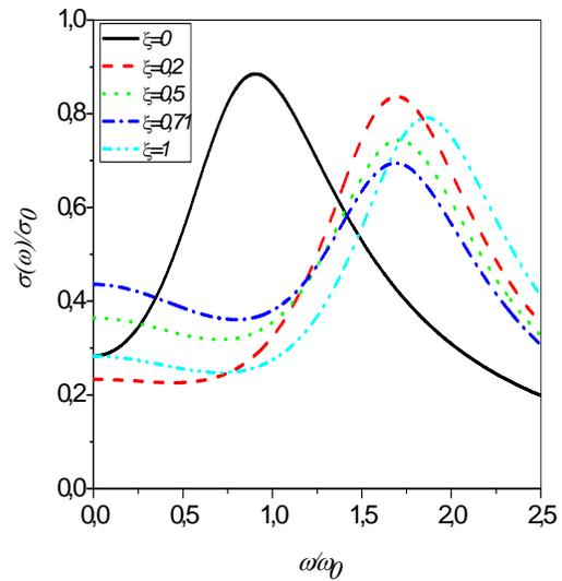
Fig. 5. Dependence of dynamic conductivity  $\sigma(\omega)$  with the frequency  $\omega$  for different values of  $\xi$ . The other parameters are  $\Gamma=7$ ,  $T=300$  K,  $V_1=0.1$  eV.
