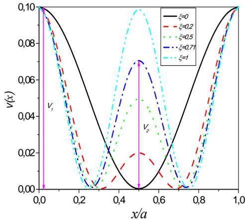
Fig. 1. Structure of the symmetric bistable potential  $V(x)$  for different values of the ratio of two potential barriers  $\xi$ .
