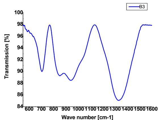
Fig. 4. FTIR spectra of sample B3.
