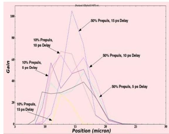
Fig. 4. Temporal evolution of the gain in plasma for the case using two pulses (black curve) and the case using three pulses where the delay between the main pulses is 5, 10 or 15 ps.
