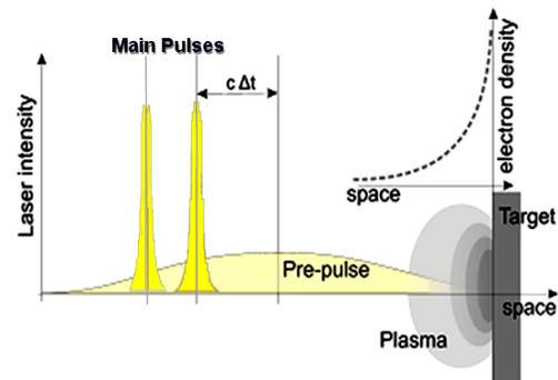
Fig. 1. Schematic representation of the proposed TCE XRL: laser pulses intensities, the target and the plasma electron density are represented in the spatial extension.
