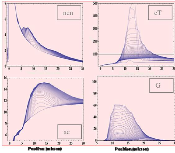
Fig. 3. Spatial and temporal evolution of the plasma parameters (electron density, electron temperature, average ionization state and the gain) for the case using one main pulse.
