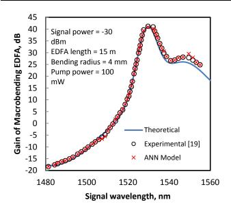
Fig. 3. Gain spectra with macro-bending effect. The input signal and pump powers are fixed at -30 dBm and 100 mW, respectively.
