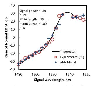
Fig. 4. Gain spectra without the macro-bending effect. The input signal and pump powers are fixed at -30 dBm and 100 mW, respectively.
