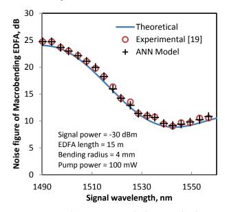
*Fig. 5.* Noise figure spectra with the macro-bending effect. The input signal and pump powers are fixed at -30 dBm and 100 mW, respectively.
