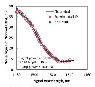
Fig. 6. Noise figure spectra without the macro-bending effect. The input signal and pump powers are fixed at -30 dBm and 100 mW, respectively.
