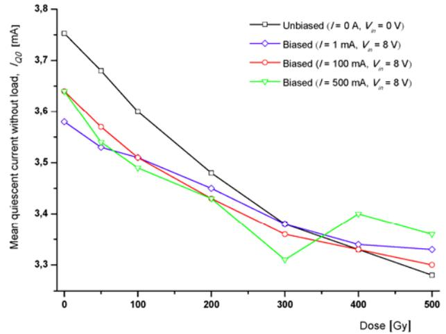
Fig. 6. Change in the mean quiescent current in the unloaded voltage regulator L4940V5 under the influence of  $\gamma$ -radiation ( $V_{in} = V_{CE(100\text{ mA})} + 4.9\text{ V}$ ,  $I_{out} = 0\text{ A}$ ).
