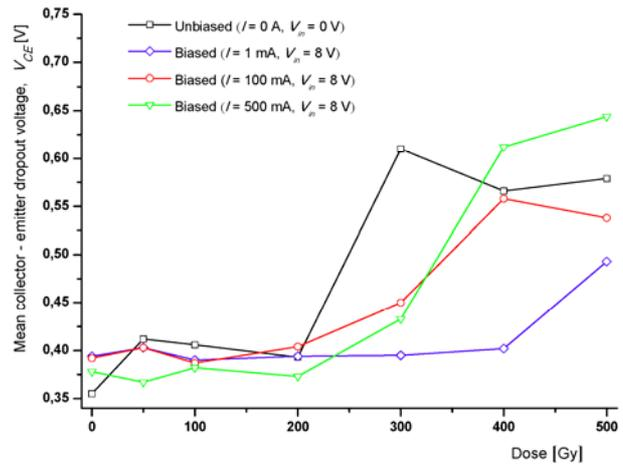
Fig. 2. Change in the mean serial transistor's minimum dropout voltage in the voltage regulator L4940V5 under the influence of  $\gamma$ -radiation ( $V_{out} = 4.9$  V,  $I_{out} = 100$  mA).
