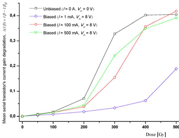
Fig. 4. Change in the mean serial transistor's current gain degradation in the voltage regulator L4940V5 under the influence of  $\gamma$ -radiation ( $V_{out} = 4.9\text{ V}$ ,  $I_{out} = 100\text{ mA}$ ).
