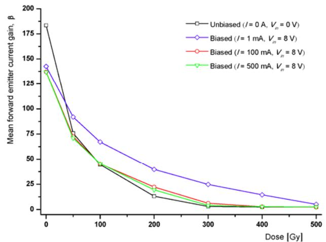
Fig. 3. Change in the mean serial transistor's forward emitter current gain in the voltage regulator L4940V5 under the influence of  $\gamma$ -radiation ( $V_{out} = 4.9$  V,  $I_{out} = 100$  mA).
