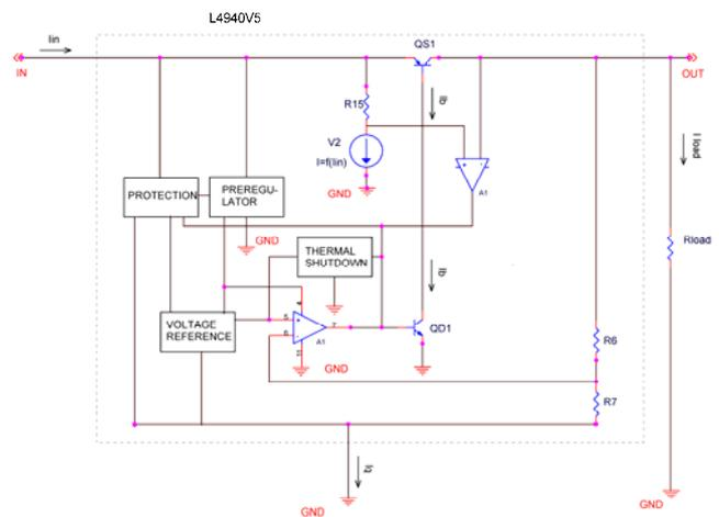
Fig. 1. Schematic block diagram of the voltage regulator "STMicroelectronics" L4940V5.
