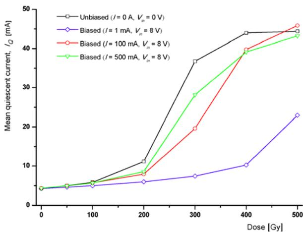
Fig. 5. Change in the mean quiescent current in the voltage regulator L4940V5 under the influence of  $\gamma$ -radiation ( $V_{out} = 4.9\text{ V}$ ,  $I_{out} = 100\text{ mA}$ ).
