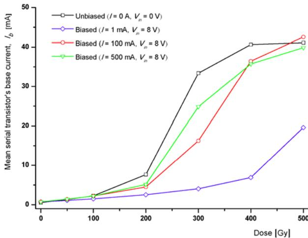
Fig. 7. Change of mean serial transistor's base current in the voltage regulator L4940V5 under the influence of  $\gamma$ -radiation ( $V_{out} = 4.9$  V,  $I_{out} = 100$  mA).
