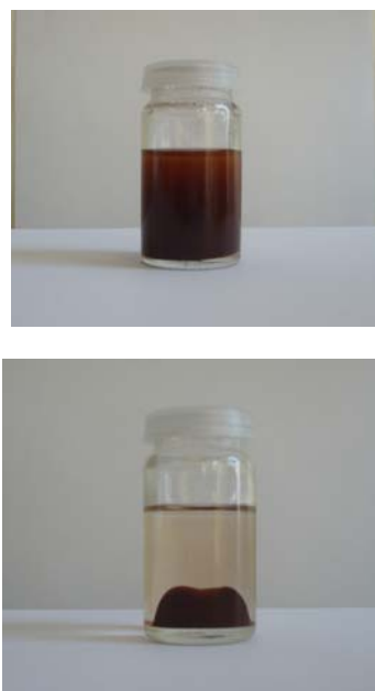
Fig. 9. The magnetic polymer particles in absence of magnetic field (first image) and in presence of magnetic field generated by a laboratory magnet (second image).
