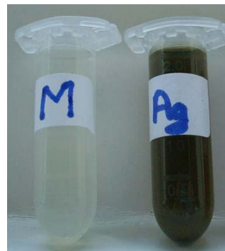
Fig. 2. Colours of 10^{-3} M \text{AgNO}_3 solution (M) and of silver nanoparticles geranium extract solution (Ag)
