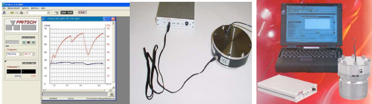
Fig.4. The evolution of temperature and pressure inside the bowl for 3 cycles of 5 minutes of alloying and 5 minutes break between them.
