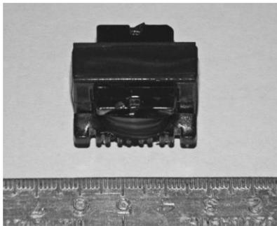
Fig. 5. Finished tapped inductor
