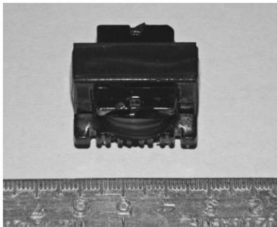
Fig. 5. Finished tapped inductor
