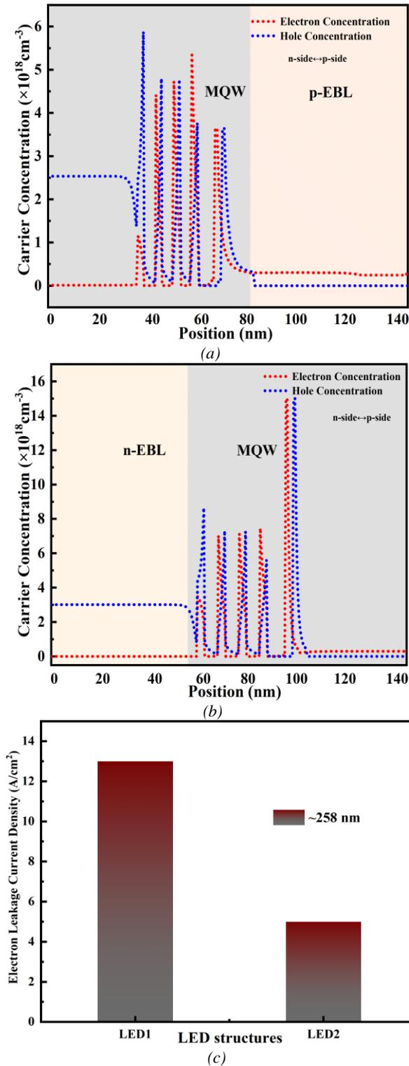
Fig. 5. Carrier concentration in the MQWs of (a) the conventional LED (LED<sub>1</sub>) and of (b) the proposed LED (LED<sub>2</sub>) at 40 mA; (c) Electron leakage current density of LED<sub>1</sub> and LED<sub>2</sub> (color online)
