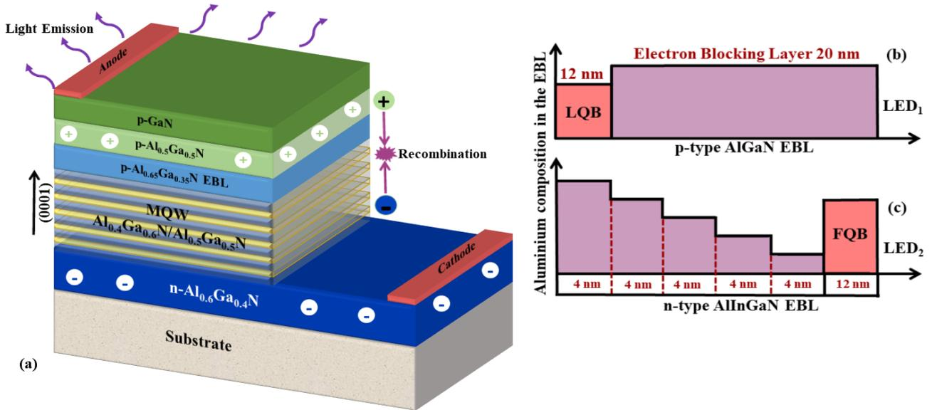
Fig. 1. (a) Schematic diagram of the conventional LED (LED<sub>1</sub>). Al composition (%) profile related to the conduction band of (b) LED<sub>1</sub> with conventional p-type AlGaN EBL and of (c) LED<sub>2</sub> with step graded n-type AlInGaN EBL with uniformly decreasing Al composition. LQB and FQB represent last quantum barrier and first quantum barrier, respectively (color online)
