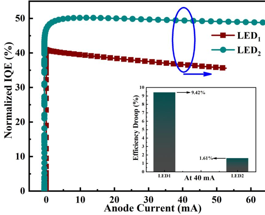
Fig. 7. IQE as a function of injected current in both LED<sub>1</sub> and LED<sub>2</sub>. Inset: Efficiency droop for each LED at 40 mA (color online)
