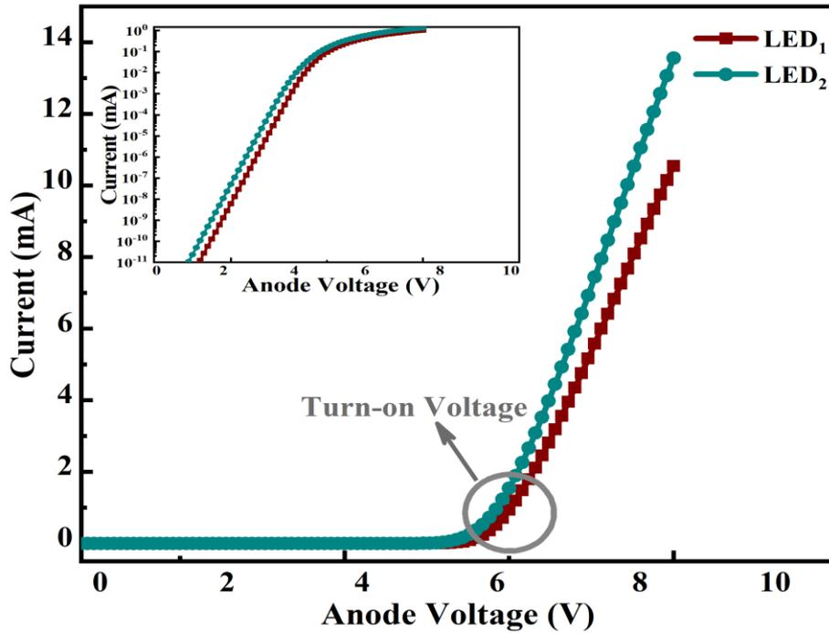
Fig. 8. I-V behaviour of both LED<sub>1</sub> and LED<sub>2</sub> in linear scales; Inset: Re-plotting of the I-V curves in a semi-log scale (color online)
