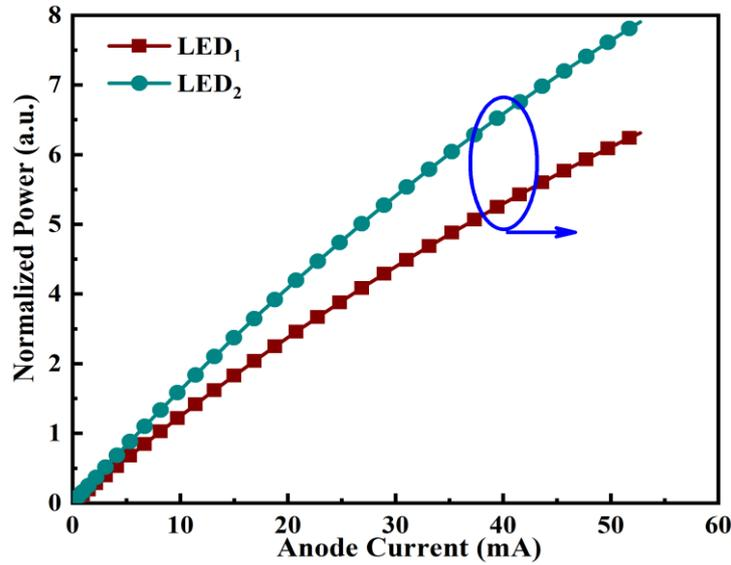
Fig. 9. Output power of both LED<sub>1</sub> and LED<sub>2</sub> as a function of injection current (color online)
