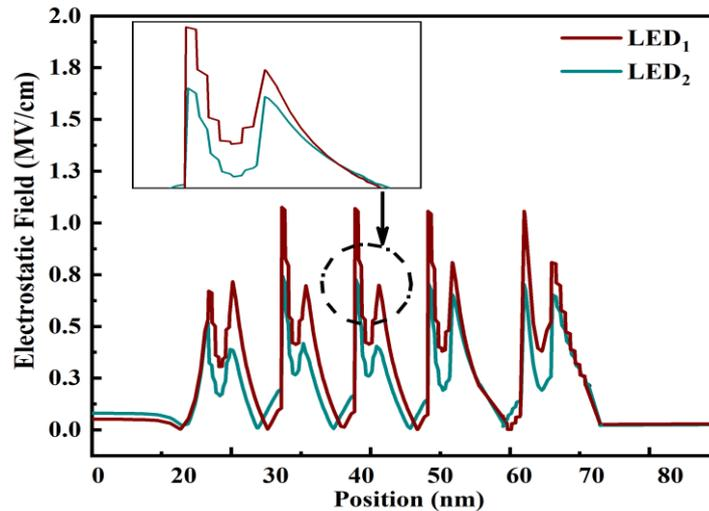
Fig. 10. Magnitude of electrostatic field in the active region of LED<sub>1</sub> and LED<sub>2</sub>; Inset: Electrostatic field in the 3<sup>rd</sup> QW (color online)
