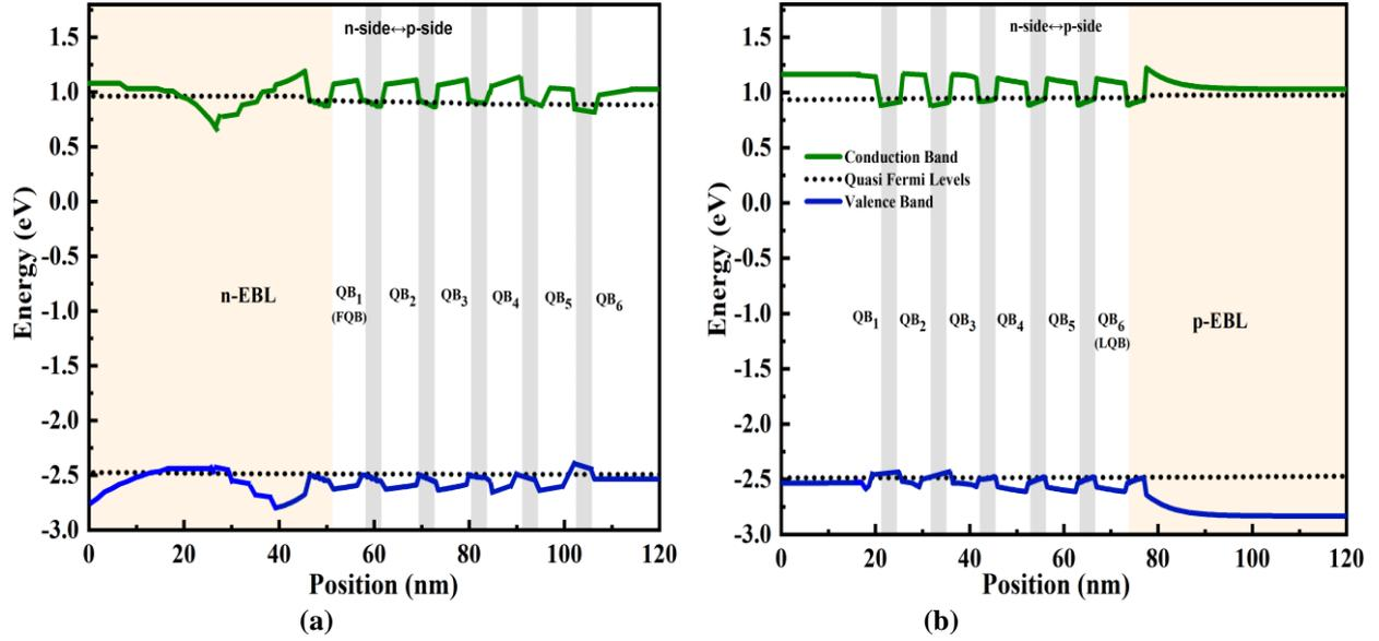
Fig. 4. Energy band profile of (a) the conventional LED ( $LED_1$ ) and of (b) the proposed LED with step-graded n-type EBL ( $LED_2$ ) at 40 mA (color online)
