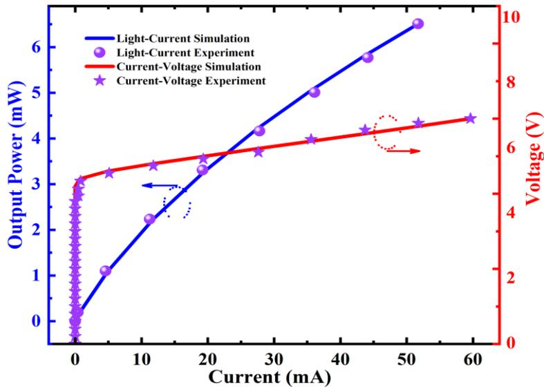
Fig. 2. Measured and calculated light-current-voltage characteristics of LED<sub>1</sub> for model validation (color online)
