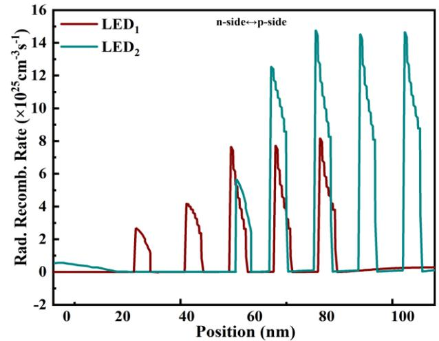
Fig. 6. Radiative recombination rate of both LED<sub>1</sub> and LED<sub>2</sub> at 40 mA (color online)
