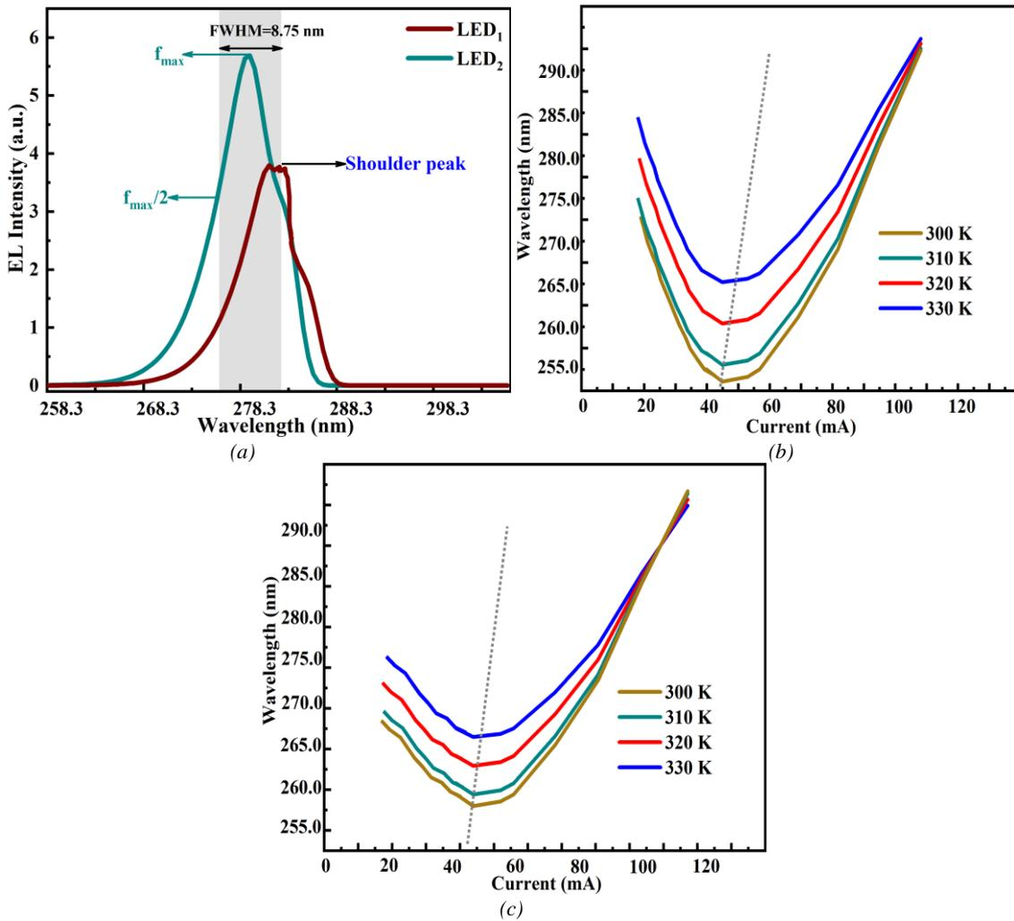
Fig. 3. (a) Electroluminescence (EL) intensity of LED<sub>1</sub> and LED<sub>2</sub> at an injection current of 40 mA, (b) Emission wavelengths as a function of injection current for LED<sub>1</sub> and (c) LED<sub>2</sub> (color online)
