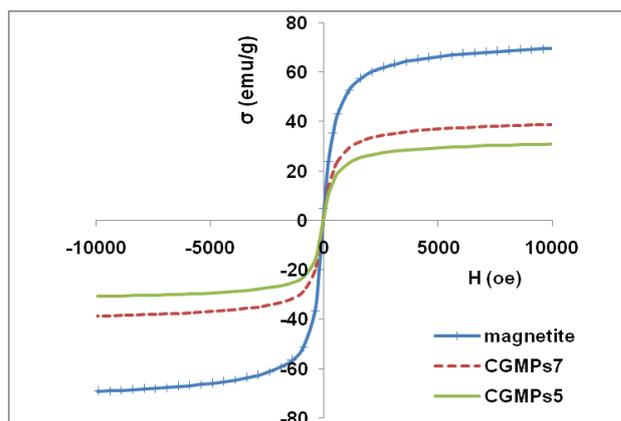
Fig. 7. Magnetizations curves for magnetite, CGMPs7 (at 1/2 polymers/magnetite ratio) and CGMPs5 (at 1/1 polymers/magnetite ratio).
