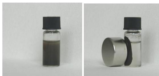
Fig. 6. The magnetic polymer particles in acetone: first image, in absence of magnetic field; second image, in presence of magnetic field generated by an external magnet.
