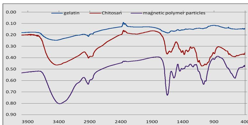
Fig. 1. The FTIR spectra for (GEL, CS) polymers and for magnetic polymer nano/microparticles, sample CGMPs1.
