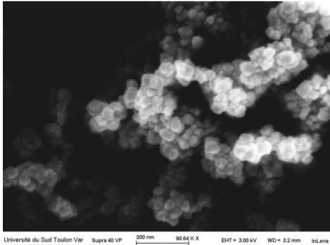
Fig. 2. The SEM microphotograph of magnetite nanoparticles (90.640 x).
