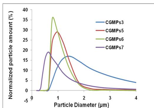
Fig. 5. Average size of magnetic polymer particles determined by diffractometry measurements.
