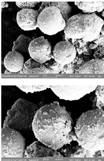
Fig. 3. The SEM microphotographs of magnetic polymer particles, sample CGMPs3 (15190 x and respectively 27480 x).
