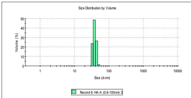
Fig. 7. HAp size distribution of nanoparticles by volume.
