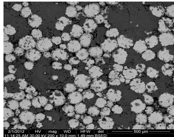
Fig. 10. SEM micrography of the composite with 70% 316L/ 30% Hap.
