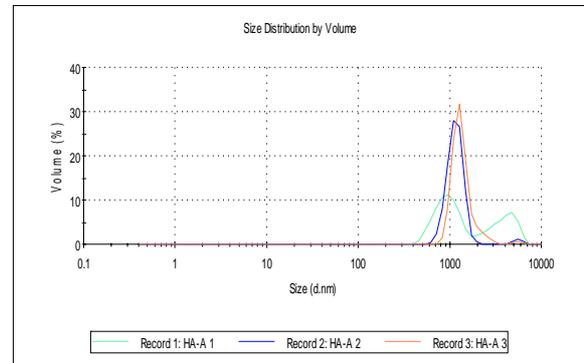
Fig. 4. Particle size distribution by volume of the 3 records.
