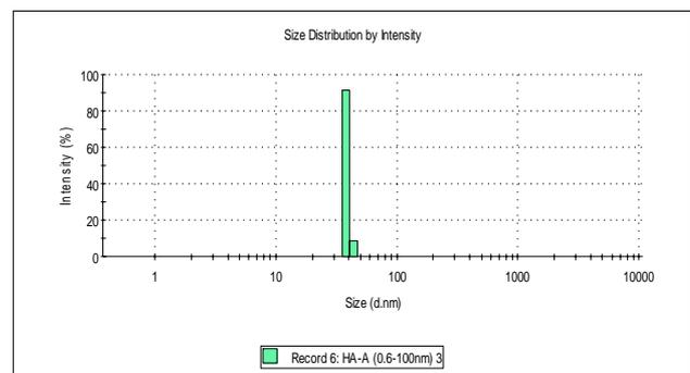
Fig. 6. HAp size distribution of nanoparticles in intensity.
