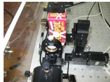
Fig.7. Photograph of emitter/detector system and X-Y sample manipulator.
