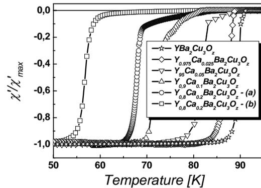
Fig. 1. Temperature dependence of the normalized real part of the fundamental AC magnetic susceptibility for all investigated samples at  $H_{ac}=1$  Oe and  $f=1000$  Hz. The maximum  $\chi_1$  value for the corresponding sample is taken for normalization.
