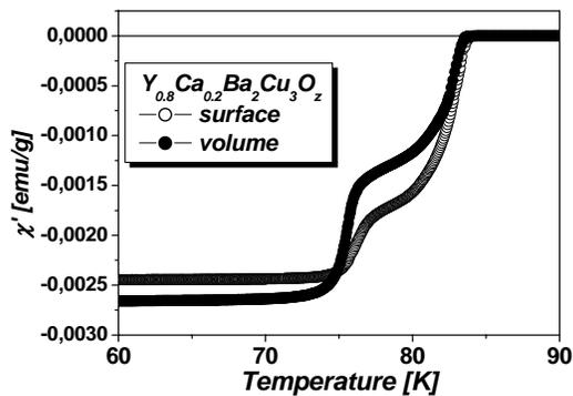
Fig. 3. Temperature dependence of the AC magnetic susceptibility for surface and volume samples at  $H_{ac}=1$  Oe and  $f=1000$  Hz.
