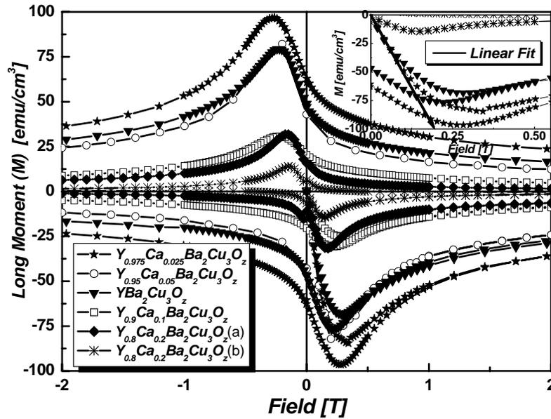
Fig. 2. Magnetization hysteresis loops for all investigated samples at 4.2 K. The inset shows the deviation from the linear fit, (which determines the  $H_{c1}$  in the case where the surface barrier is ignored). For the  $Y_{0.8}Ca_{0.2}Ba_2Cu_3O_z$ -(b) sample, the flux penetration starts immediately after the field is increased from zero.
