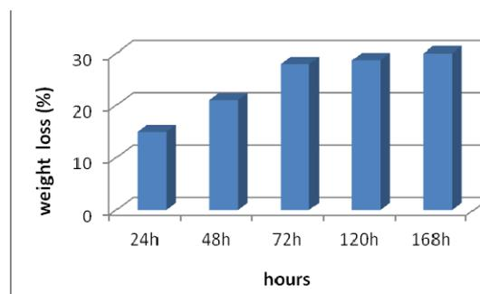
Fig. 5. Weight loss of polymeric samples after enzymatic hydrolysis.
