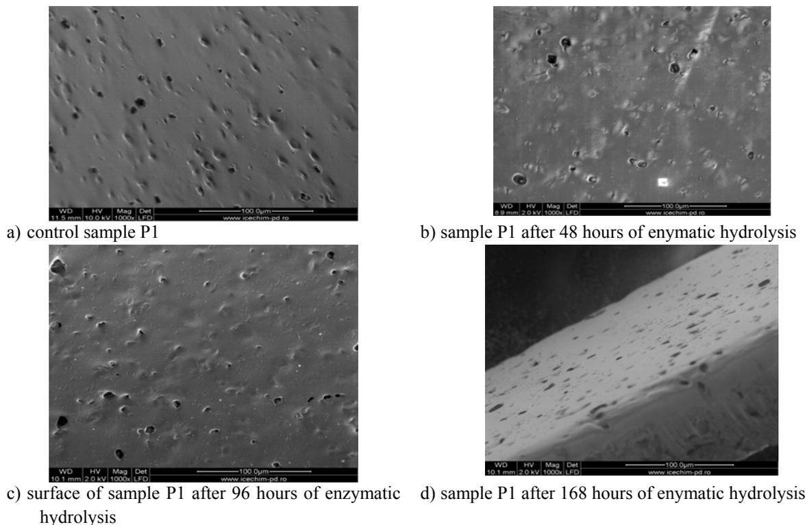
Fig. 4. SEM micrographs of the (a) control sample, (b, c and d) blends samples collected at different hydrolysis times (magnification 1000x).
