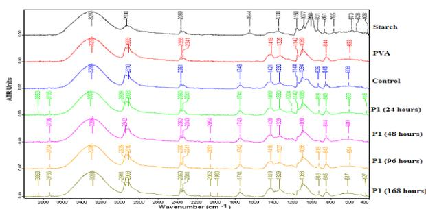
Fig. 6. ATR-FTIR spectra of the PVA/starch blends.
