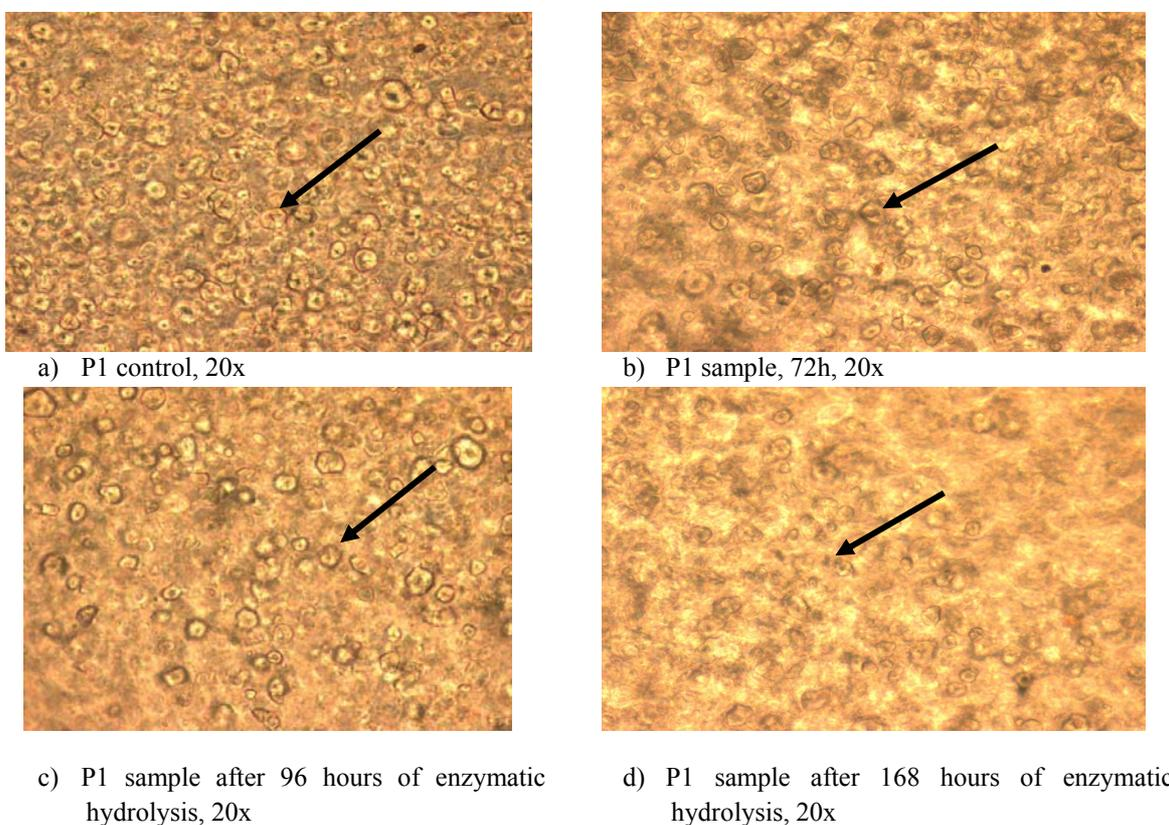
Fig. 2. Optical microscopy applied to polymeric samples after enzymatic hydrolysis with bacterial  $\alpha$ -amylase (black arrow - (starch granules).
