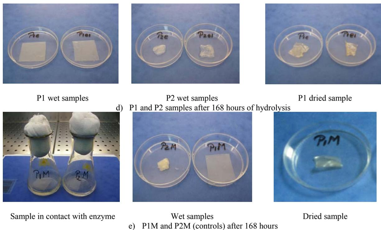
Fig. 1. Polymeric samples after enzymatic hydrolysis with bacterial  $\alpha$ -amylase at 27° C.
