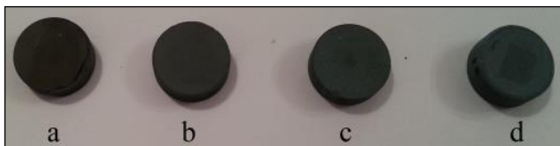
Fig. 4. Sintered compacts of Co-Cr doped with a) 5%HA b) 10%HA, c) 15%HA, d) 20%HA
