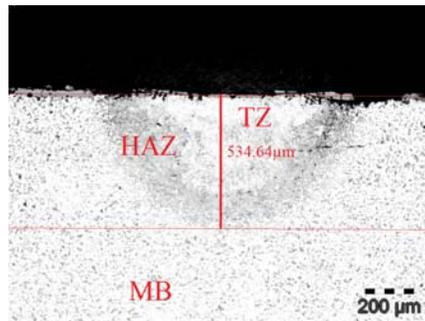
Fig. 3. Macroscopic analysis of an area treated with Nd:YAG laser, power density 8.41 kW/cm<sup>2</sup>, 100x magnitude.
