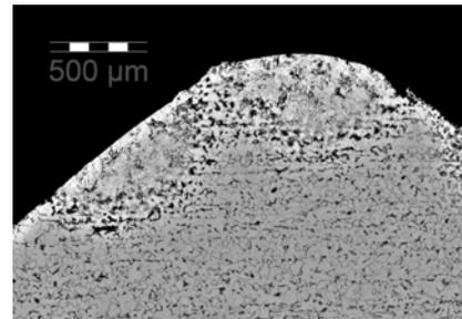
Fig. 9. The transversal section of laser heat treated zone, using a power density of 6.3 kW/cm<sup>2</sup>.
