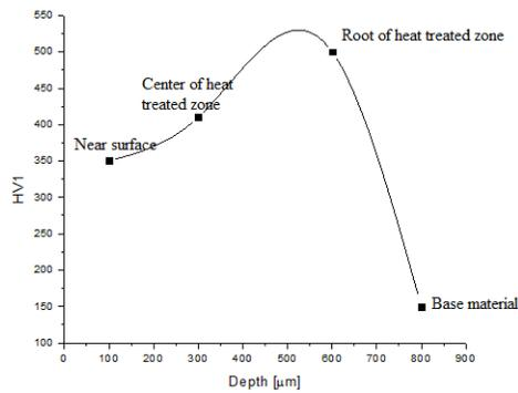
Fig. 7. Hardness evolution depending on the depth of penetration.
