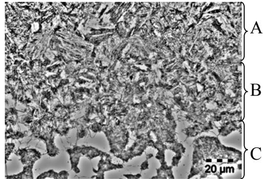
Fig. 4b. Granular structure of the material (A – fine grains in the thermal treatment zone, B – transition zone or heat affected zone – HAZ and C – base material).
