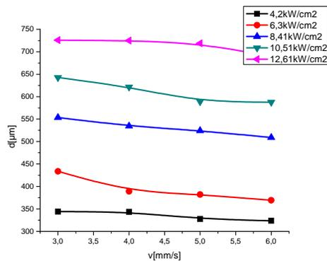
Fig. 8. Variation of heat treated zone depth depending on laser beam speed and power density.
