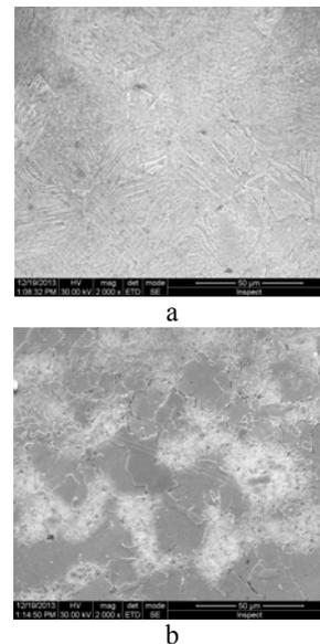
Fig. 10. Microstructure of the laser heat treated zone using power density of 6.3 kW/cm<sup>2</sup> and rotations speed of 27°/sec a) in the heat treated zone and b) in the heat affected zone.
