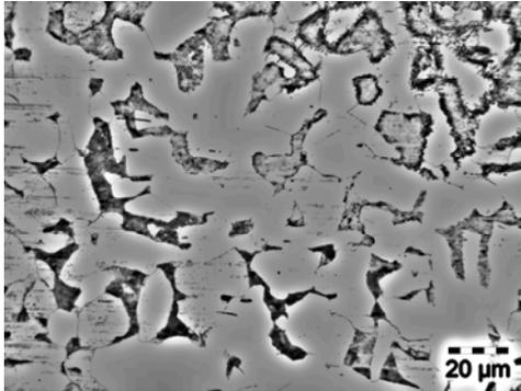
Fig. 4. Granular structure of the base material.
