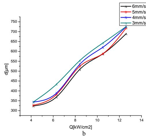
Fig. 5. Evolution of penetrations depth: a) calculated values; b) measured values as function of laser energy during laser surface treatment for different values of speed.
