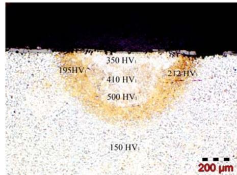
Fig. 6. Average values of microhardness in the treated area.
