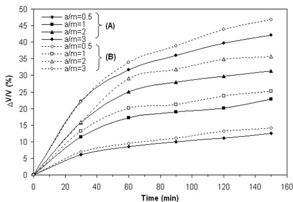
Fig.3 Variation of the volume shrinkage with the heat treatment duration for the studied samples  $Mg_{0.3}Cu_{0.2}Zn_{0.5}Fe_2O_4$  (A) and  $Mg_{0.2}Cu_{0.3}Zn_{0.5}Fe_2O_4$  (B) prepared with different  $a/m$  ratios.
