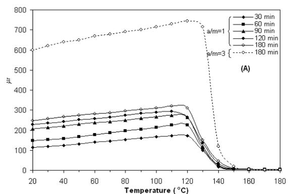
Fig.5 Variation of magnetic permeability with temperature for the sample  $Mg_{0.3}Cu_{0.2}Zn_{0.5}Fe_2O_4$  (A) prepared with the ratio  $a/m=1.3$  and with different duration of the heat treatment.
