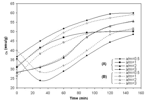
Fig.4: Variation of the saturation magnetization with the duration of the heat treatment for the studied samples  $Mg_{0.3}Cu_{0.2}Zn_{0.5}Fe_2O_4$  (A) and  $Mg_{0.2}Cu_{0.3}Zn_{0.5}Fe_2O_4$  (B) prepared with various  $a/m$ .
