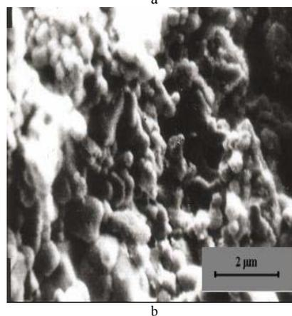
Fig. 2. SEM micrograph for two different magnifications for the  $Mg_{0.3}Cu_{0.2}Zn_{0.5}Fe_2O_4$  (A) sample, after a heat treatment of 90 minutes at  $1000^\circ C$
