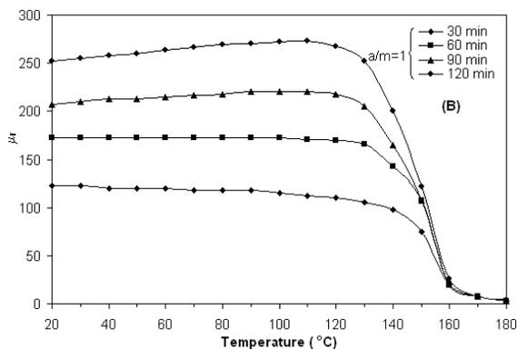
Fig. 7. Temperature variation of magnetic permeability for the sample  $\text{Mg}_{0.2}\text{Cu}_{0.3}\text{Zn}_{0.5}\text{Fe}_2\text{O}_4$  (B) prepared with the ratio  $a/m = 1$  and different heat treatment durations.
