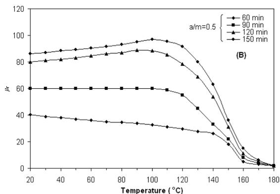
Fig. 6. Magnetic permeability variation with temperature for the sample  $\text{Mg}_{0.2}\text{Cu}_{0.3}\text{Zn}_{0.5}\text{Fe}_2\text{O}_4$  (B) prepared with the ratio  $a/m=0.5$  and different durations of the heat treatment
