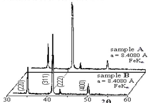
Fig. 1 X-ray diffractograms for  $Mg_{0.3}Cu_{0.2}Zn_{0.5}Fe_2O_4$  (A) and  $Mg_{0.2}Cu_{0.3}Zn_{0.5}Fe_2O_4$  (B) samples treated for 60 minutes at  $1000^\circ C$
