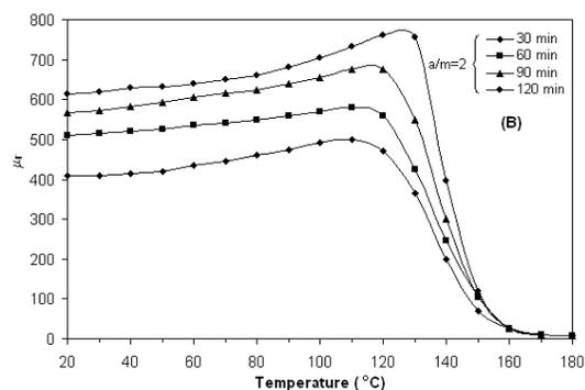
Fig. 8. Magnetic permeability variation with temperature for the sample  $\text{Mg}_{0.2}\text{Cu}_{0.3}\text{Zn}_{0.5}\text{Fe}_2\text{O}_4$  (B) prepared with the ratio  $a/m = 2$  and with different heat treatment durations.
