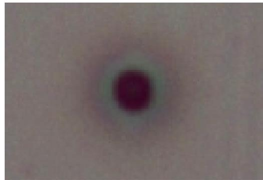
Fig. 5. Pattern of the dark spot after light exposure of amorphous  $(As_4S_3Se_3)_{0.93}Sn_{0.07}$  thin films with beam laser ( $\lambda=532.18$  nm,  $P=1$  mW).
