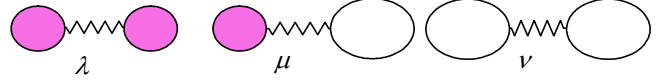
Fig. 1 Elastic constants corresponding to the spin state of the nearest neighbor pair of atoms (LS in pink and HS in white).
