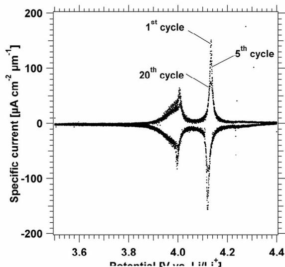
Fig. 3. Typical cyclic voltammogram in 1M LiClO<sub>4</sub>/PC electrolyte at 0.05 mV s<sup>-1</sup> of a Li<sub>1+x</sub>Mn<sub>2</sub>O<sub>4-δ</sub> thin film deposited on uncoated glassy carbon.
