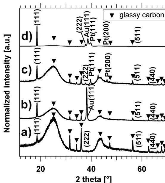
Fig. 1. X-ray diffraction patterns of  $\text{Li}_{1+x}\text{Mn}_2\text{O}_{4-\delta}$  thin films (a) on glassy carbon, (b) on Au coated glassy carbon, (c) on Pt coated glassy carbon, and (d) on Au/Pt coated glassy carbon substrates. The reflexes of the glassy carbon are marked with ▼.
