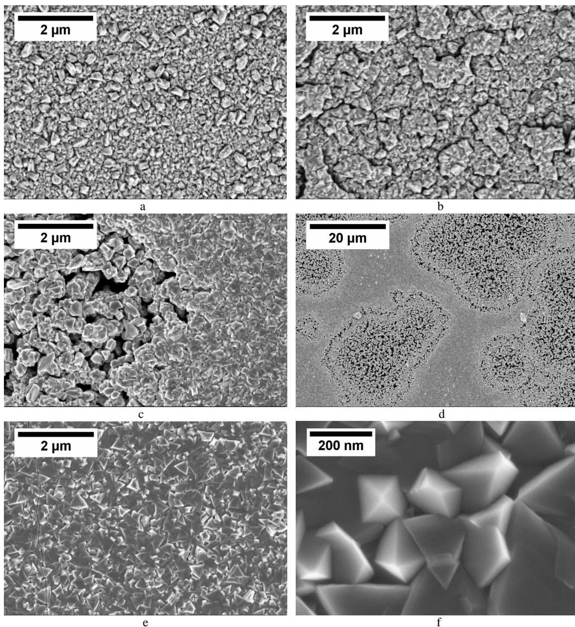
Fig. 2. SEM images of thin  $\text{Li}_{1+x}\text{Mn}_2\text{O}_{4-\delta}$  films deposited (a) on glassy carbon, (b) on Au coated glassy carbon, (c-d) on Pt coated glassy carbon, and (e-f) on Au/Pt coated glassy carbon substrates.
