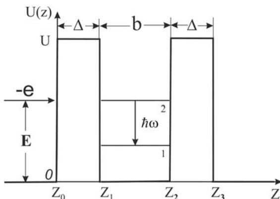
Fig. 1. Energy scheme for the electrons and geometry of two-barrier RTS.
