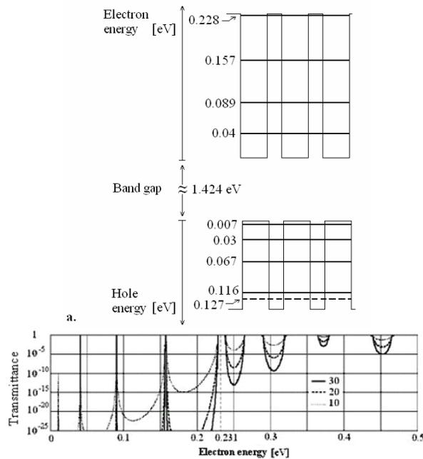
Fig. 1. (a) Schematic representation of levels in the valence bands and conduction for the MQW system  $Al_{0.3}Ga_{0.7}As/GaAs$  containing 30 quantum wells. The corresponding level for the heavy gaps it's made with dotted line. (b) Transmission coefficient based on the electron energy for the same system. The curves parameter is the number of quantum wells.
