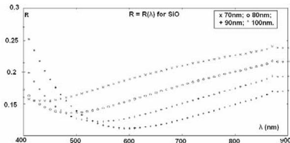
Fig. 3. Simulation of the reflectance for a solar cell with QW structure, for a SiO anti reflecting coating.
