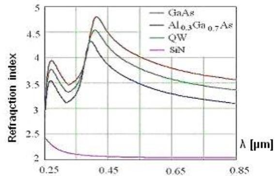
Fig. 4. The refraction index for the materials involved in constructing a MQW cell.
