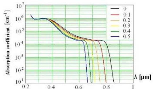
Fig. 7. Absorption coefficient of Al<sub>x</sub>Ga<sub>1-x</sub>As depending on wavelength;  $x$  is the curves parameter.
