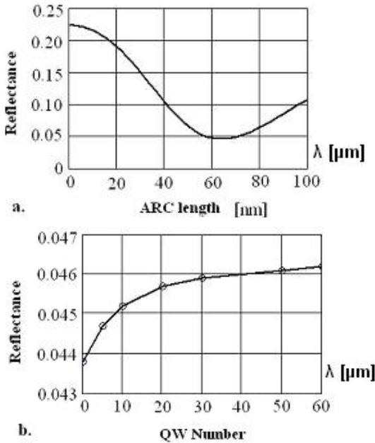
Fig. 6. (a). ARC length influence over the cell reflectance; (b). Influence of the number of quantum wells over the cell reflectance. The HM model was run for GaAs/Al<sub>0.3</sub>Ga<sub>0.7</sub>As with  $N_w = 30$ ,  $l_w = 20\text{ nm}$  and  $l_b = 10\text{ nm}$ .
