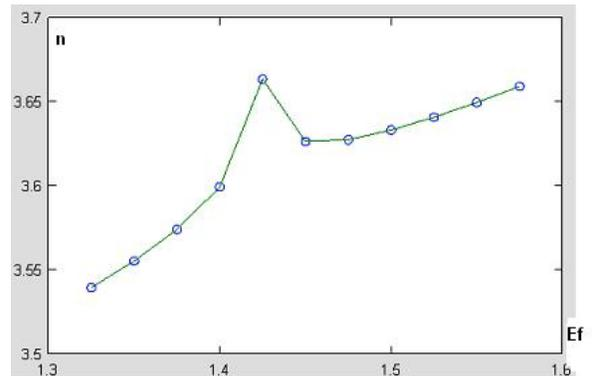
Fig. 2. The refraction index of the cells with quantum wells depending on the photon energy.
