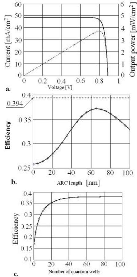
Fig. 9. (a) Voltage-current characteristic (line) and the output power (points) of the cell with the following MQW system: GaAs/ $Al_{0.3}Ga_{0.7}As$ ,  $N_w = 30$ ,  $l_w = 20$  nm,  $l_b = 10$  nm and the anti reflecting coating depth  $d = 64$  nm. (b) The MQW cell efficiency depending on the anti reflecting coating depth. The dotted line indicates the ideal cell efficiency with zero reflectance. (c) The efficiency of MQW cell based on the number of quantum wells.
