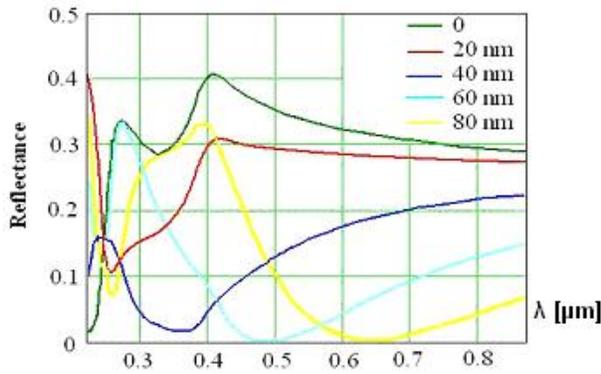
Fig. 5. Spectral reflectance of the MQW cell for different width (in nanometer) of the anti reflecting coating. The HM model was run for GaAs/Al<sub>0.3</sub>Ga<sub>0.7</sub>As with  $N_w = 30$ ,  $l_w = 20\text{nm}$  and  $l_b = 10\text{nm}$ .
