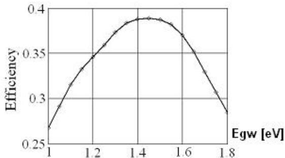
Fig. 10. The MQW cell efficiency depending on the width of the band gap of the material in which are located the quantum wells.
