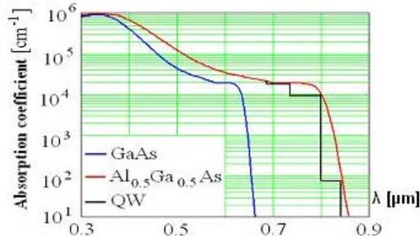
Fig. 8. The absorption coefficient in GaAs crystal, the ternary compound  $Al_{0.5}Ga_{0.5}As$  is calculated using axes translation in MQW system.
