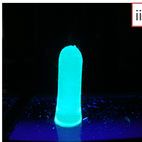
Fig.1. i) XRD patterns of original Si NCs powder and ii). NCs Si doped sol gel rod (8 month latter) under UV lamp.
