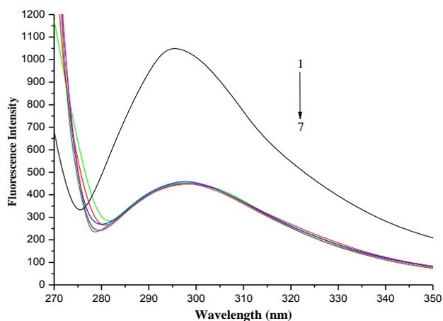
Fig. 1. The fluorescence spectra of  $4.8 \times 10^{-2} \text{g} \cdot \text{L}^{-1}$  keratin induced by  $4.1 \times 10^{-11} \text{mol} \cdot \text{L}^{-1}$  silver nanoparticles at pH 7.2 at different reaction time 1 - 0s, 2 - 30s, 3 - 6min, 4 - 15min, 5 - 30min, 6 - 60min, 7 - 120min
