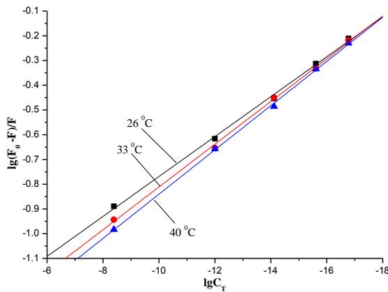
Fig. 5. The relationship between the fluorescence intensity and the concentration of silver nanoparticles at pH 7.5.
