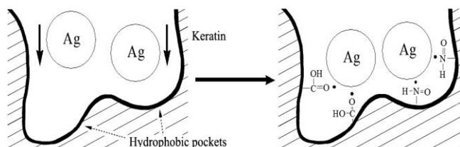
Fig. 6. The pictorial description of the reaction between keratin and silver nanoparticles.
