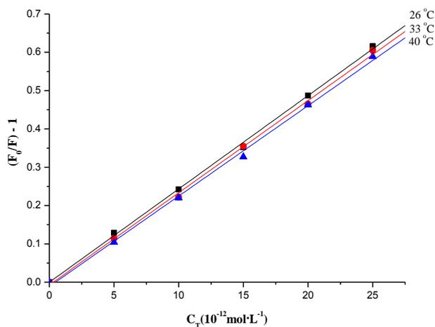
Fig. 4. The Stern-Volmer relationship between the concentration of silver nanoparticles and relative fluorescence intensity of keratin at different temperatures.
