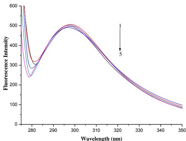
Fig. 2. The fluorescence spectra of  $5.0 \times 10^{-2} \text{ g} \cdot \text{L}^{-1}$  keratin induced by  $4.1 \times 10^{-11} \text{ mol} \cdot \text{L}^{-1}$  silver nanoparticles at different pH values 1 - 5.5, 2 - 6.5, 3 - 7.0, 4 - 7.5, 5 - 8.5.
