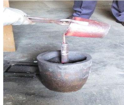
Fig. 4. Stirring of Molten metal.
